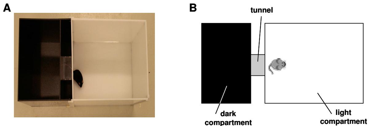
**Figure 3.6** Light-dark box test
