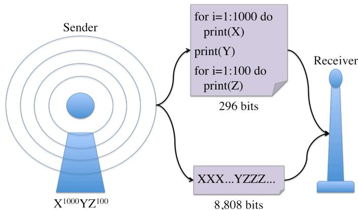
Figure 2.1: An intuitive example of the Minimum Description Length principle. Sending the string message  $X^{1000}YZ^{100}$  from a sender to a receiver as simple string would require 8,808 bits. Transferring the same string coded by the coding schemata shown on top only 296 bits are required, therefore, a total of 8,512 bits can be saved.
