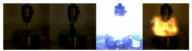
Figure 2.76. High Speed Video Images (4000 frames per second) of the electrostatic ignition of BTAT and subsequent explosive decomposition. The four pictures show the unreacted sample, ignition of the sample by electrostatic discharge accompanied by formation of dark coloured gases, detonation accompanied by a flash of light and burning of the hot decomposition gases (from left to right).
