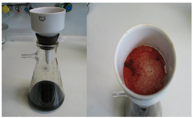
1) The residue was dissolved in acetonitrile (20 mL) and filtered to remove unreacted starting material (3,6-diamino-1,2,4,5-tetrazine, 200mg).
