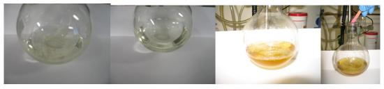
**Figure 2.114.** Trinitroethanol (left picture), colourless solution of trinitroethanol and ethyl chlorothioformate (second left picture). A vigorous reaction starts immediately after the addition of iron(III)chloride (picuture in the middle). The formation of hydrogen chloride can be monitored using indicator paper (right picture).
