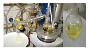
Figure 2.115. Destillation of S-ethyl-2,2,2-trinitroethyl-thioformate (left picture) and pure product (right picture).
