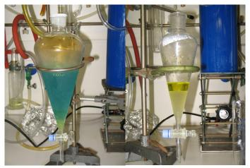
Figure 2.27. Isolation of Tetranitromethane. The reaction mixture is poured onto ice water and separates as heavy phase (left picture). NMR pure tetranitromethane is obtained as a colourless liquid after several washings using sodium bicarbonate (right picuture).
