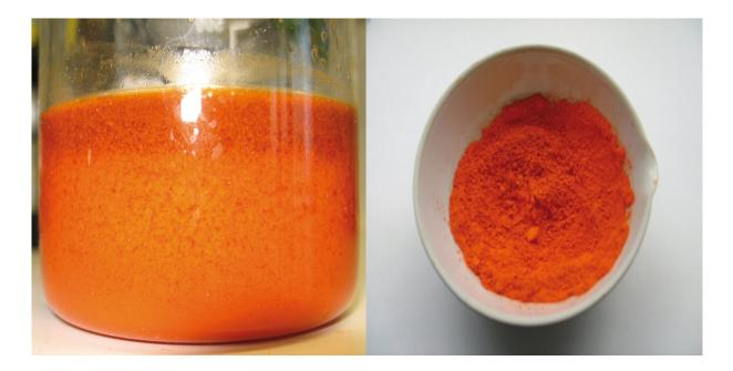
7) Hydrochloric acid (2M) is added to precipitate the BTAT from solution. Finally, the product is filtered and washed with water yielding BTAT as bright orange powder of high purity.
