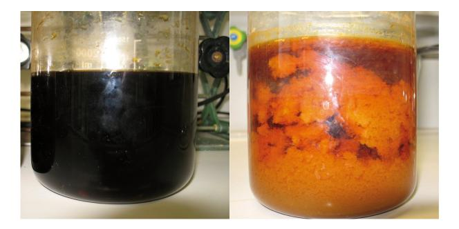
2) Hydrochloric acid (2M, 2L) was added to the filtrate to precipitate the BTAT from solution and keep the iron complex in solution. It takes several hours for the product to precipitate (bright orange colour). The picture on the right was taken after one day.
