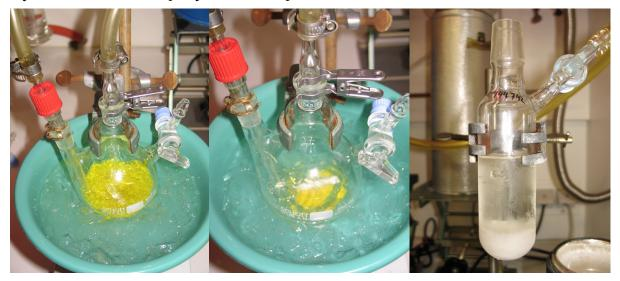
Figure 2.28. Synthesis of trinitromethane from potassium nitroformate. Dry potassium nitroformate is suspended in pentane and acidified using gaseous hydrochloric acid (left picture) affording a colourless solution of trinitromethane in pentane after a few minutes. On passing a stream of nitrogen over the pentane solution, trinitromethane precipitates from the solution in high yield and purity (right picture).
