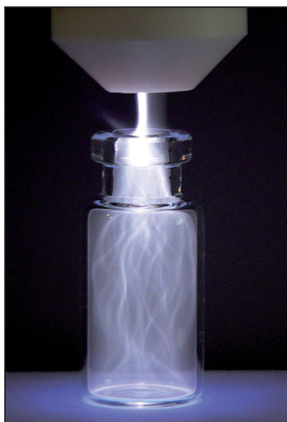
Figure 2: Surface treatment process of 2R borosilicate glass vials with argon plasma.
