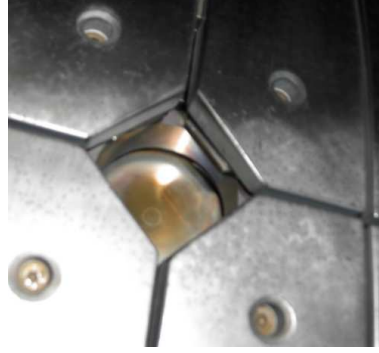
Figure 4.10: A photograph of an in-vessel mirror at the inner column of the ASDEX Upgrade plasma vessel. The diameter of the mirror is about 5 cm. It is surrounded by the tungsten-coated first wall carbon tiles.
