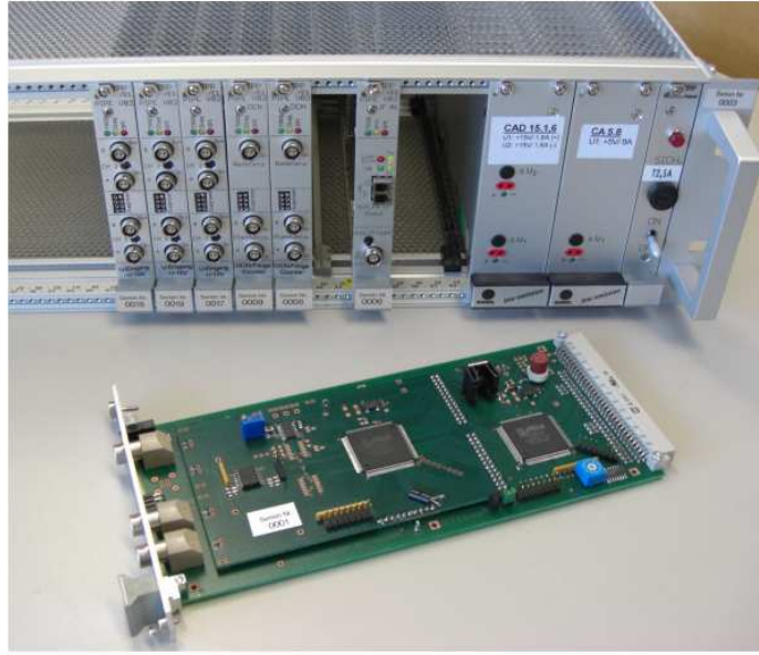
Figure 5.18: A photograph of the CPLD based phase counter in front of the crate with the backplane bus system.
