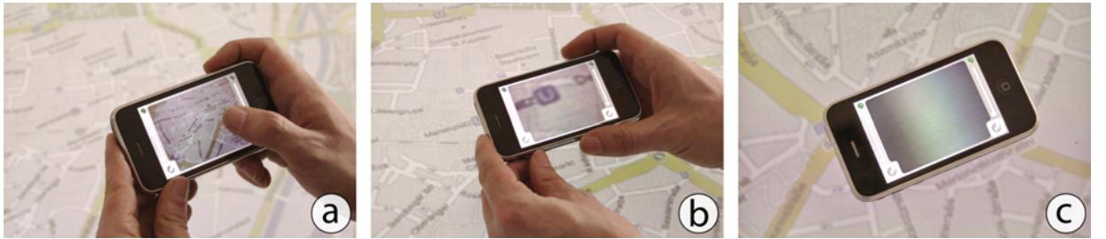
**Figure 8.6:** Problems of live video with directly superimposed displays: (a) At distances of several inches users can interact in a sharp video image. (b) Getting closer blurs the video image. (c) Placing the camera on the external screen makes the video unusable.
