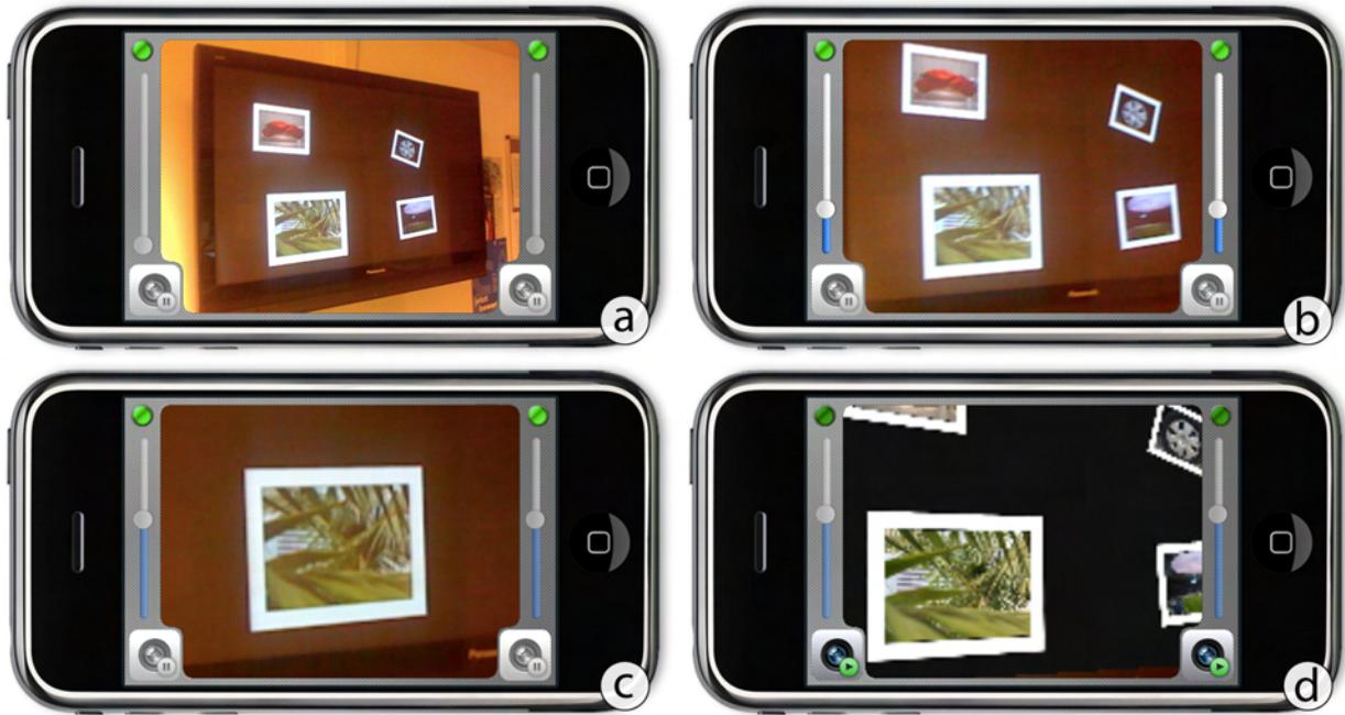
**Figure 7.13:** The four *Touch Projector* interfaces used during the study: (a) Original camera interface. (b) Manual zoom capabilities. (c) Automatic zooming. (d) Freezing the camera image with temporary overlay for precise interaction.
