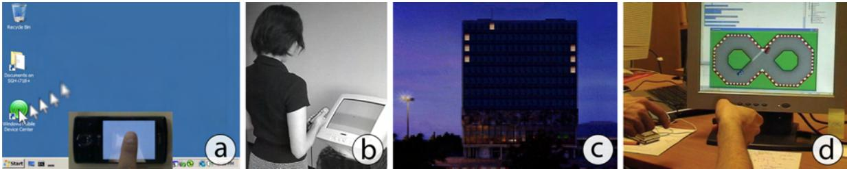
**Figure 2.10:** Pointing at a distance using mobile devices: a) *ARC-Pad* allows absolute and relative positioning on remote displays [MI09]. b) A user controlling a remote pointer with an isometric joystick [SMK01]. c) The project *Blinkenlights* allows users to play the classic pong on building facades using the keypad of a mobile device [Met01]. d) The device's accelerometers can be used to control virtual cars on a larger display [VCBE08].
