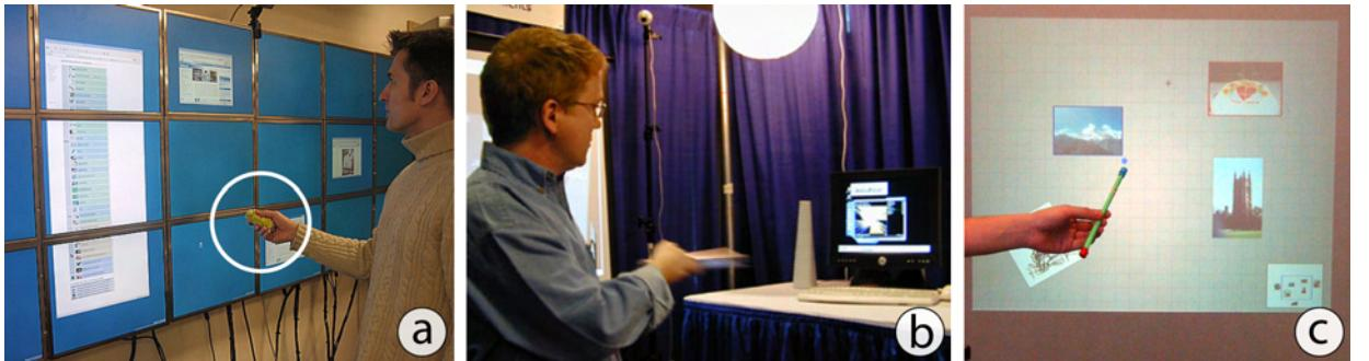
**Figure 2.7:** Controlling a pointer on distant displays: a) *Soap* controls a mouse pointer in mid-air [BSW06]. b) The *XWand* can be used to point at distant screens further allowing gestures to control the content [WS03]. c) *VisionWand* uses two cameras to detect both ends of the wand to obtain its position and orientation [CB03].
