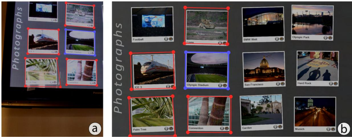
**Figure 5.5:** Matching the location of detected items (red) relative to the reference item (blue). Left shows the taken image and right shows the predicted positions based on the reference item. Although the lower right item is off by several pixel, the system can still match it according to its position. However, the detection shows errors which does not allow for taking the reference item to compute the final transformation matrix.
