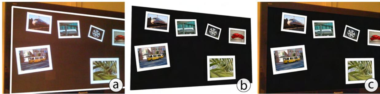
**Figure 7.11:** Overlaying the paused video image for permanent feedback: (a) The paused video image (white borders denote the detected screen). The correctly distorted overlay (b) is then overlaid and permanently updated on the paused image (c).
