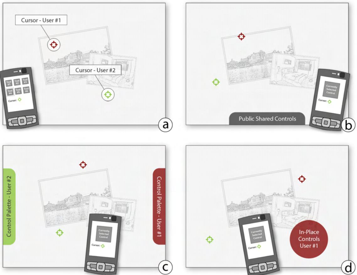
**Figure 4.9:** The four different tool palette placements: (a) depicts the *ultra-private* controls entirely displayed on the mobile device. (b) shows the *shared* tool palette accessible by every user. (c) denotes the *personal* tool palettes displayed on the public display. (d) shows a recently "called" *temporal-personal* menu (here by user #1).
