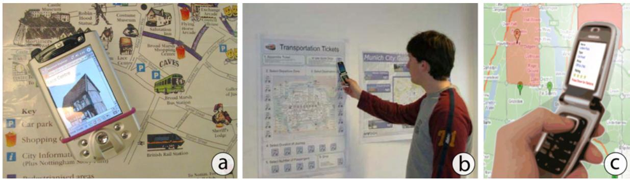
**Figure 2.9:** Touching displays physically for interaction: a) *Marked-up maps* allow mobile devices to display digital content associated to a position on the map [RRA<sup>+06</sup>]. b) A user *collects* data from a poster [BHP<sup>+08</sup>]. c) Multiple tags with a front projection to allow for two-dimensional input [HR08].
