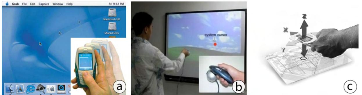
**Figure 2.11:** Relative and absolute pointing with the mobile device's camera: a) *Sweep* uses optical flow analysis turning the mobile device into a mouse-like interface [BRS05]. b) With *Direct Pointer*, users point at the position on the target display in an absolute fashion [JOMS06]. c) Optical tracking can be used to determine the mobile device's position and orientation with 6 degrees of freedom [HELO05].
