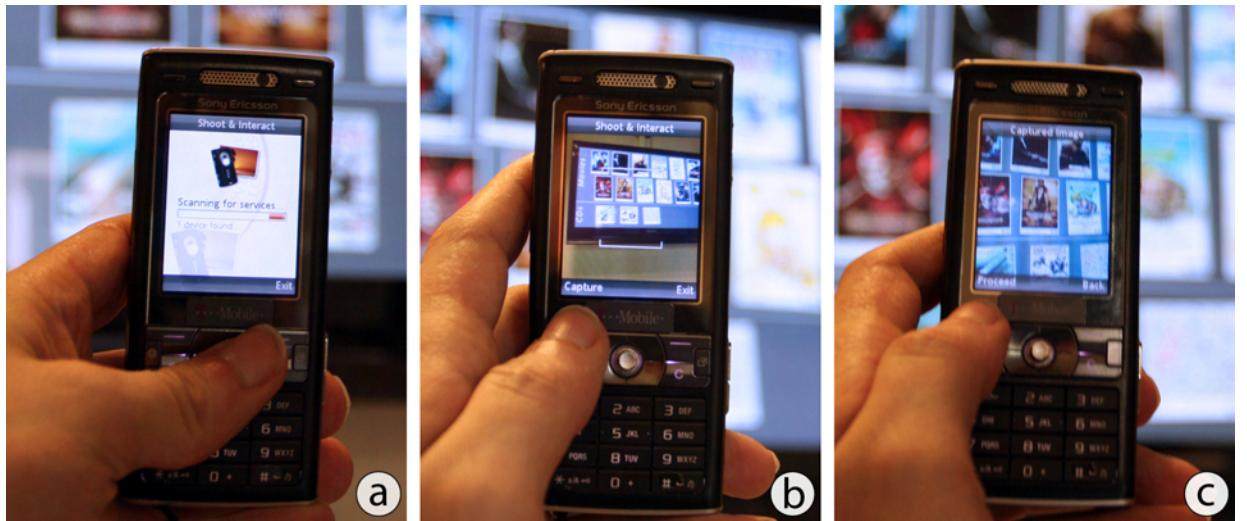
**Figure 5.7:** Connecting and selecting content *through the display*: While the application launches, the system connects to the display already with a specialized service name (a). Then the camera preview is shown which allows users to aim at content of interest (b). After capturing an image, users can decide whether this image has the content in its center (c).
