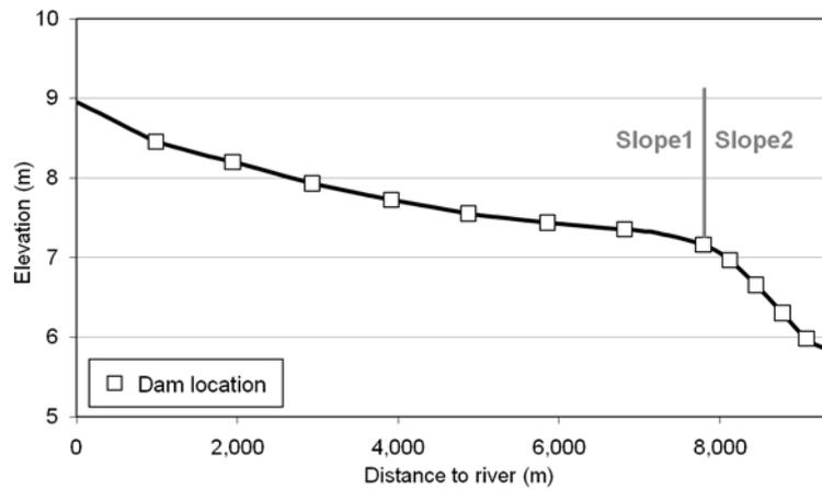
**Fig. 7** Slope of the peat surface next to a canal in Bangah catchment as measured in the modelled DTM (0 marks the most upstream part of the canal). 13 dams are required to reduce large scale drainage.
