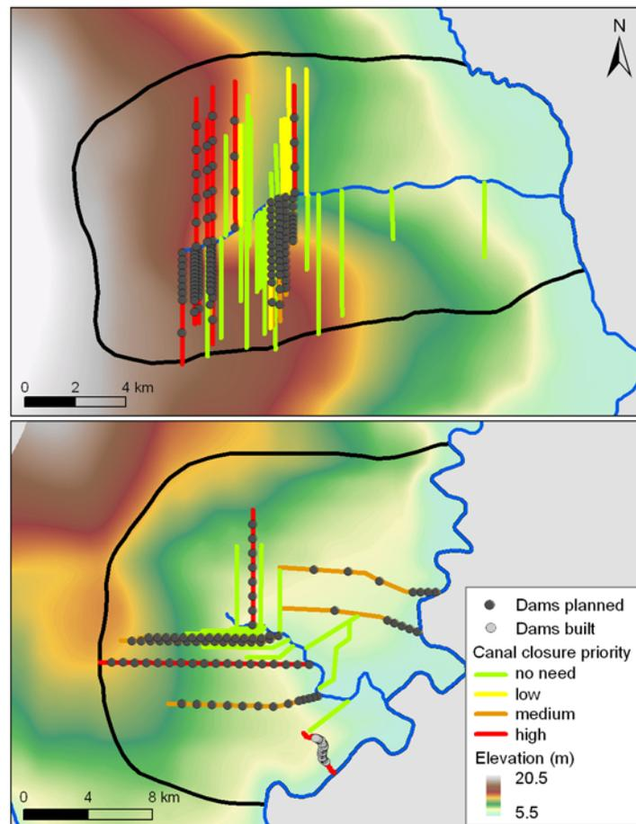
**Fig. 8** Location of dams to be constructed for an efficient reduction of drainage in the Bakung and Bangah catchments. Only canals ranked as medium and high priority should be closed. Data are superimposed on the peat surface DTM.
