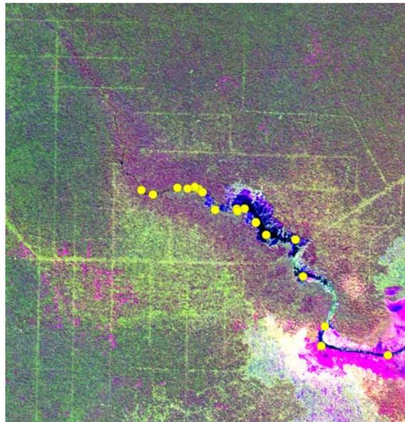
**Fig. 6** SPOT satellite image from May 2004 showing the course of canals and railway tracks in the Bangah catchment as bright green lines as well as sites of illegal logging (pink and bright green “dots”). The origin of drainage canals recorded during field work is superimposed as yellow dots.
