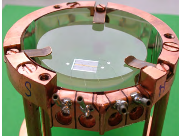
Figure 7.1: Photograph of detector CaMoO 4 -1 mounted in the holder for the transition measurements. The bond wires for the electrical contacts to the readout circuit are visible.
