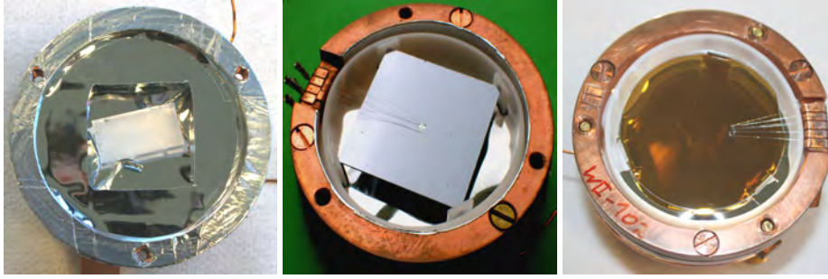
Figure 6.2: Left: (20 \times 10 \times 5) mm 3 CaMoO 4 sample mounted in a holder. The crystal is held by two pairs of copper clamps covered with an aluminum tape. Middle: Silicon light detector BE11 mounted in a copper holder which is surrounded by a teflon ring. The detector is held by four thin teflon pegs. Right: Silicon-on-sapphire light detector HANS mounted in a copper holder which is also surrounded by a teflon ring. The detector is held by three copper clamps covered with a layer of sputtered aluminum. The bond wires for the electrical contact are visible.
