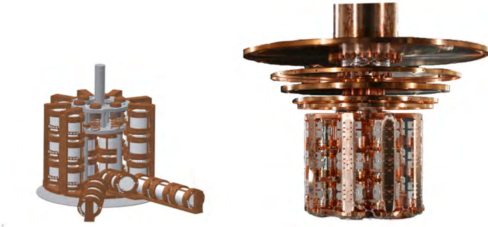
Figure 2.5: Left: Drawing of the detector support structure. Detector modules are mounted on towers which can be handled as a whole. Right: Photograph of the carousel equipped with the detector modules for the Run 31. The top parts of the five thermal shield are visible.
