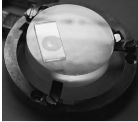
Figure 7.4: Photograph of the \text{ZnWO}_4 -1 crystal with a \text{ZnWO}_4 wafer glued onto its surface with help of Araldite 2011 glue after the low temperature test.
