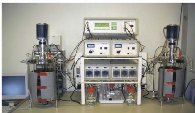
**Figure 2: Dual -vessel (2x10l) laboratory fermenter system for mass culture of *M. gryphiswaldense***
