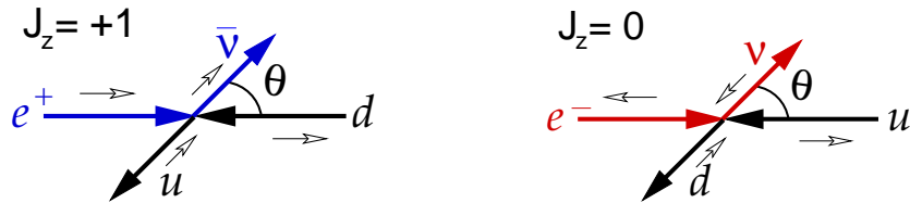
Figure 1.7: Illustration of the angular dependence in charged current reactions (in the CM frame, assuming the z direction along the e^\pm motion and \theta being the scattering angle of the \nu ): (left) the angular momentum component J_z is not conserved if the \bar{\nu} is scattered backwards, i.e. the interaction amplitude is proportional to (1 - \cos \theta) ; (right) the interaction amplitude does not depend on \theta because J_z = 0 .
