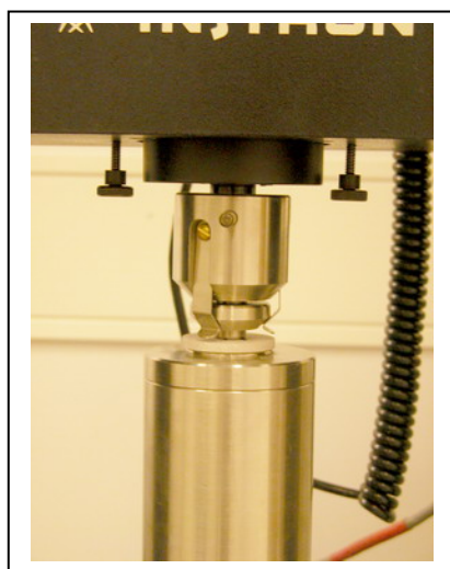
Figure 24. Picture and schema of the biaxial flexural strength set up.
