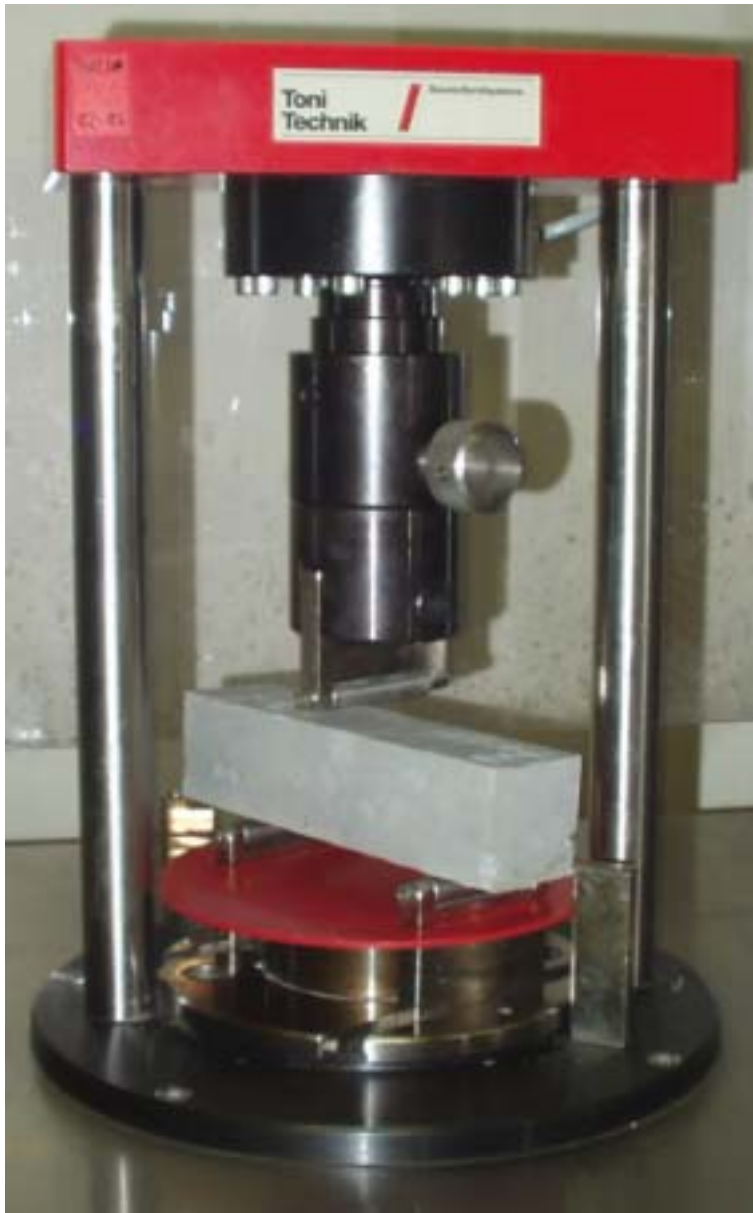
Figure 23: Device as used for the static fragmentation tests with Mr. W. Bögl of the Materialprüfungsamt in Munich. The sample is placed on two static bearing edges and loaded by a hydraulically controlled punching tool from above. (picture credit: Wolfgang Bögl)
