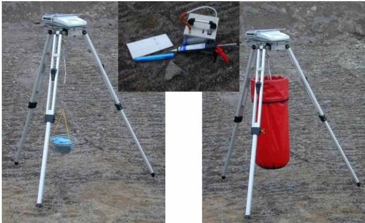
Figure 12: The set-up for the density measurements directly in the field. The balance is fixed on the tripod. A water reservoir (right) is placed below the balance and the sample can be submerged with a special holding device (left). The inset shows the vacuum pump, the silicon injection device and plastic bags.
