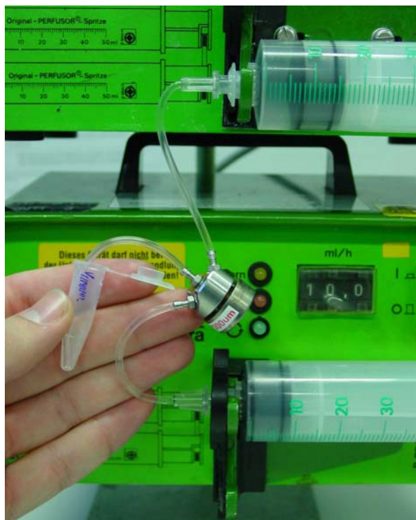
Figure 4-8: Experimental setup with micromixer ® : two syringe pumps feed the micromixer ® with a constant, pulsation-free flow of the protein and the precipitation solution, laminar mixing and precipitation is performed within the device, thus forming the microparticles.
