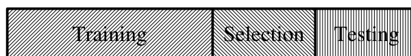
Figure 3.13: Usually the available examples should be split up into three sets: the training set is used to train the statistical learning method, the selection set is used to choose the optimal generalisation behaviour among different parameter settings, and the test set provides an independent estimate for the true performance. The splitting could typically be 50%:25%:25%.
