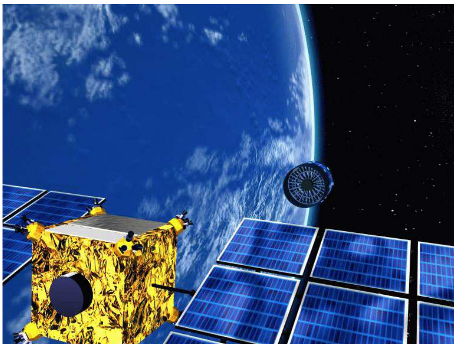
Figure 2.33: The XEUS satellite with its two components (mirror spacecraft and detector spacecraft) in an artist's view.
