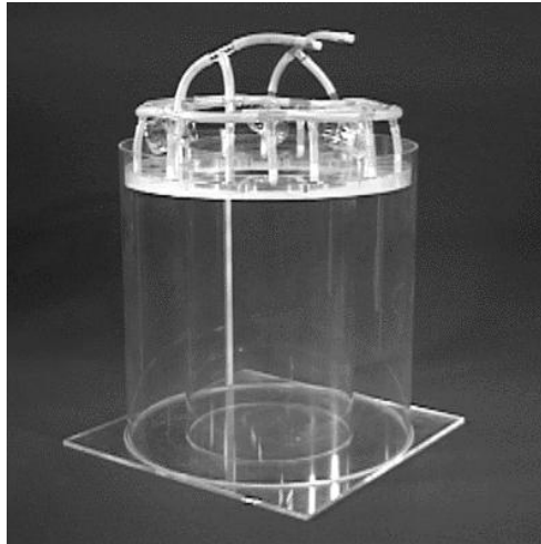
Figure 1.2: A picture of the cylindrical annulus used for the QBO experiments at the university of Kyoto ( www.gfd-dennou.org , 2004). In the picture the oscillating membrane can be seen at the top of the annulus, while in the original experiment of Plumb and McEwan the membrane was mounted at the bottom.
