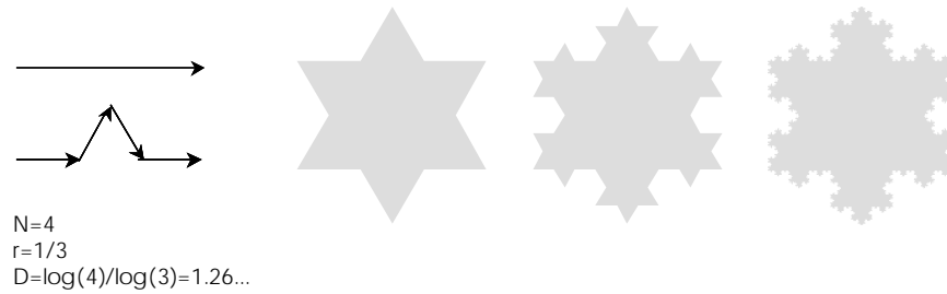
Figure 6.24: Recursive replacement procedure for generating the von Koch snowflake curve (left) and the snowflake for one, two and five iteration steps.
