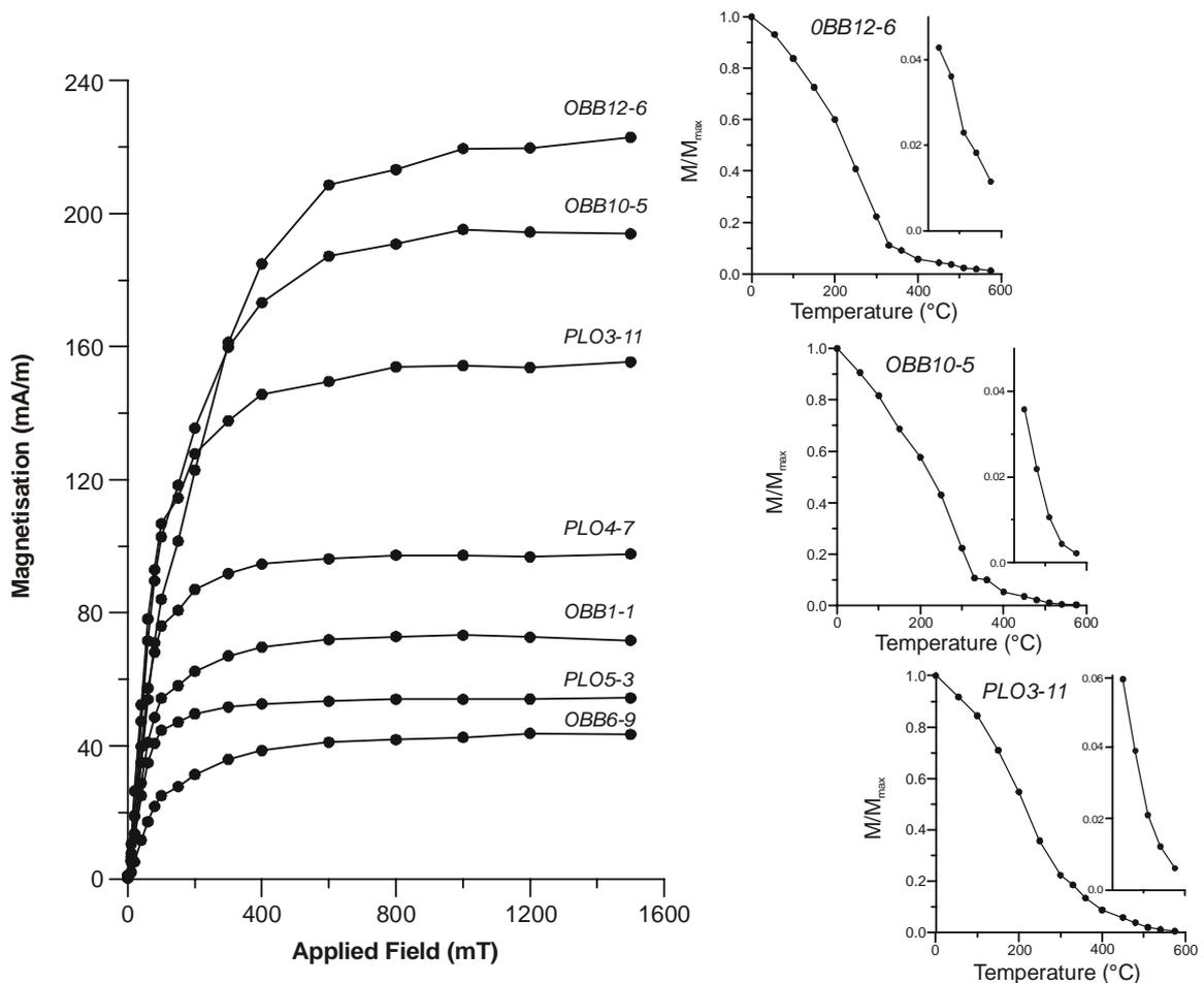
Figure 4-15: Acquisition curves of a monidirectional isothermal remanent magnetization (IRM) of Lower Devonian sediments of the central Carnic Alps and thermal demagnetisation curves.
