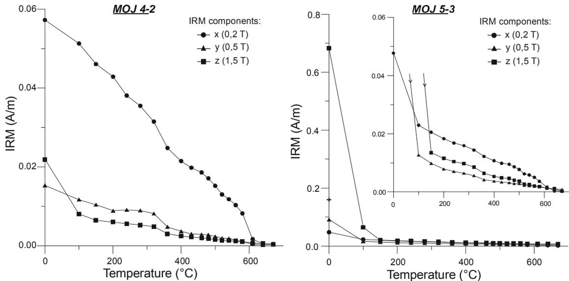
Figure 5-3: Thermal demagnetisation of triaxial differential IRM (method described in [Lowrie, 1990]) in (a) of specimen MOJ4-2 and in (b) of specimen MOJ5-3. The blow-up in 5-3(b) shows a detail of the demagnetisation curve.
