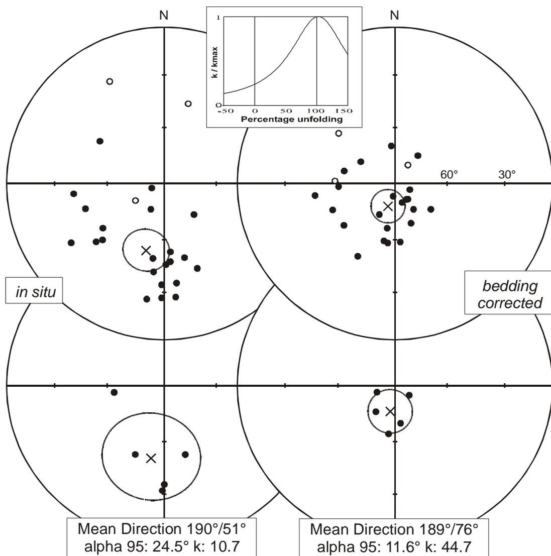
Figure 3-3: Equal area stereographic projections of the Early Ordovician sample (top) and site mean (bottom) C magnetisation before and after structural correction, and the  $k/k_{max}$  ratios versus percentage unfolding. Solid (open) circles represent lower (upper) hemisphere projections;  $k$  is the precision parameter [Fisher, 1953], and alpha 95 is the cone of 95% confidence.
