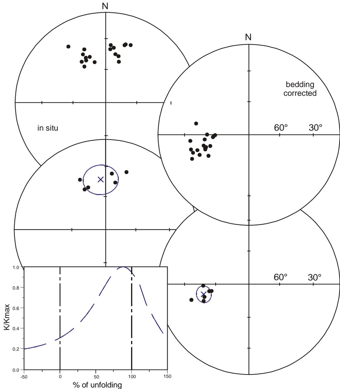
Figure 4-13: Equal area stereographic projections of the Early Devonian sample (top) and fold section mean (bottom) C1 magnetisation before and after structural correction, and the  $k/k_{max}$  ratios versus percentage of unfolding. Solid (open) circles represent lower (upper) hemisphere projections;  $k$  is the precision parameter [Fisher, 1953], and  $\alpha_{95}$  is the cone of 95% confidence.
