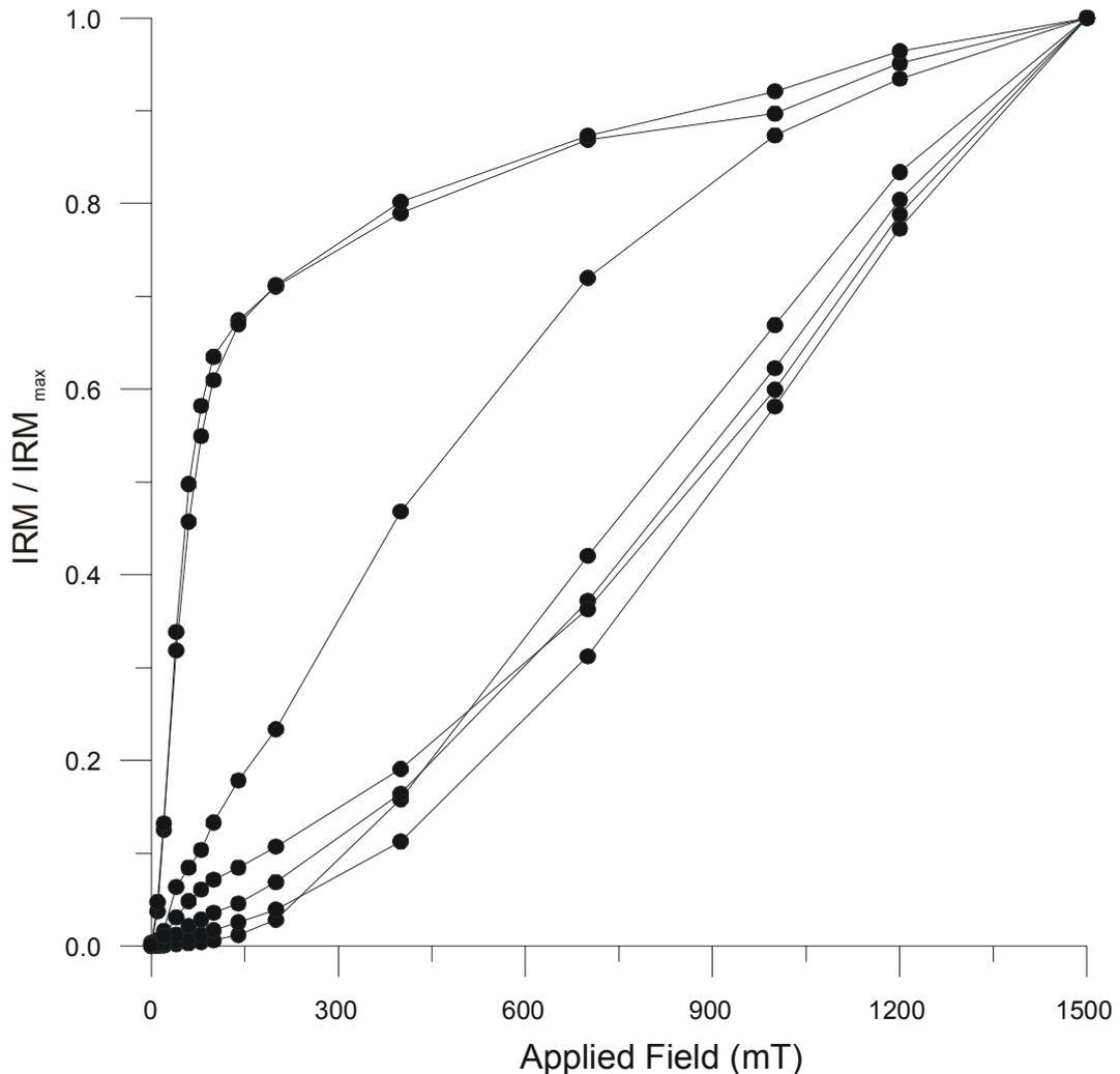
Figure 5-2: Normalized acquisition curves of monodirectional isothermal remanent magnetisation (IRM) of Ordovician limestones of the Mojca quarry.
