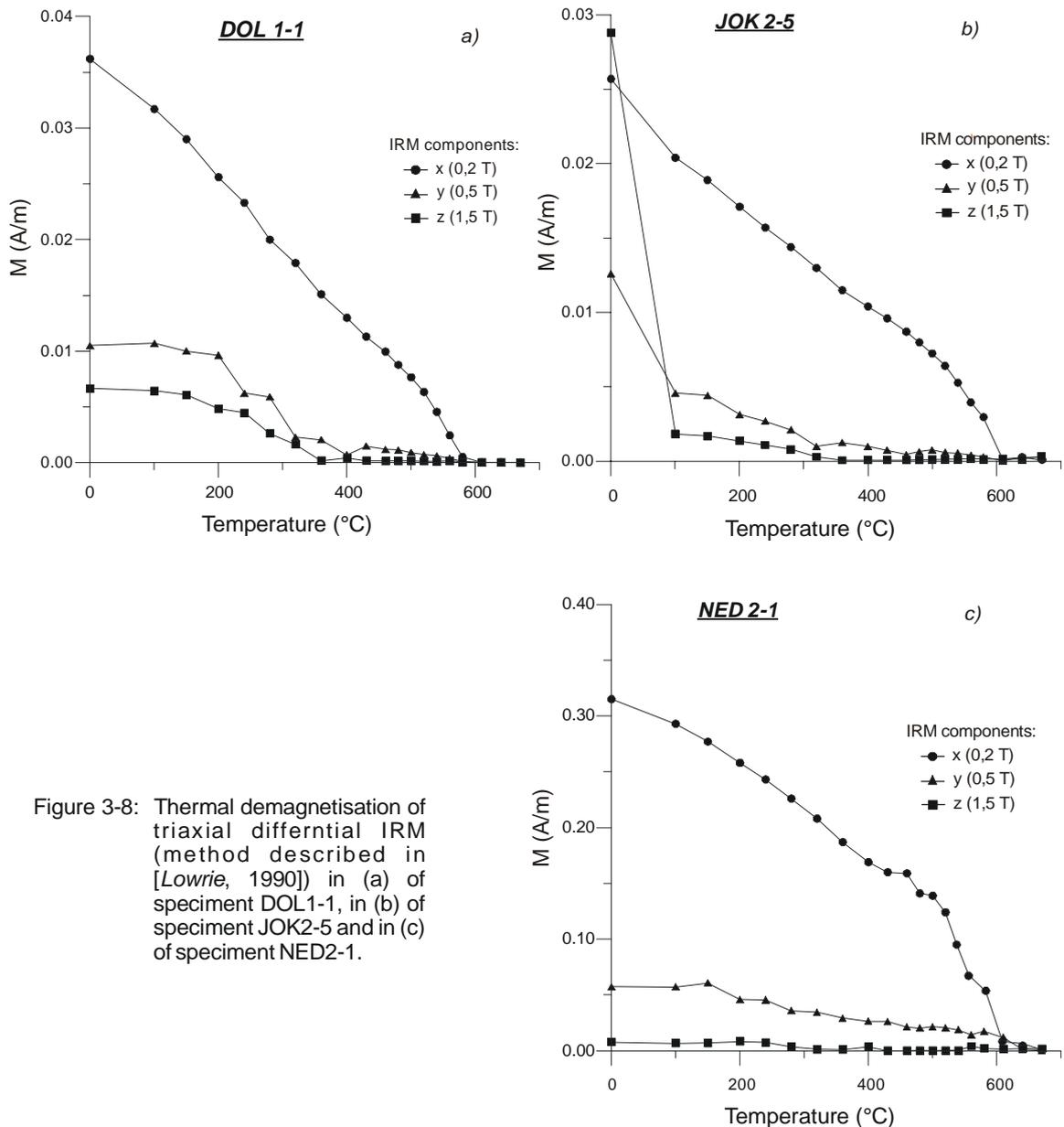
Figure 3-8: Thermal demagnetisation of triaxial differential IRM (method described in [Lowrie, 1990]) in (a) of specimen DOL1-1, in (b) of specimen JOK2-5 and in (c) of specimen NED2-1.
