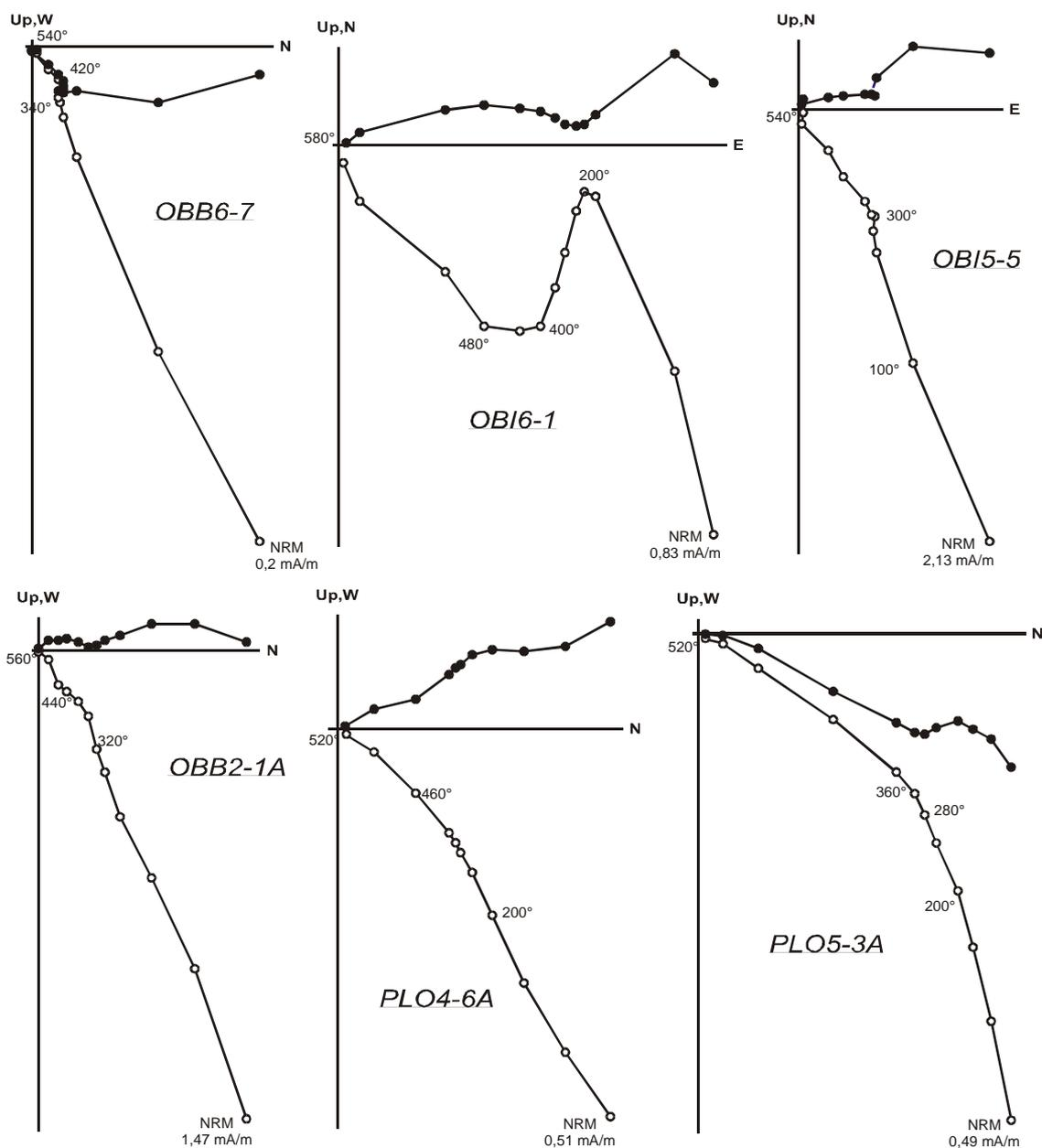
Figure 4-12: Orthogonal projection of thermal demagnetization data for samples from the Lower Devonian carbonates. All directions are plotted in in situ coordinates. Notation as in Fig. 4-4. Almost all Samples show a removal of component A up to 200°-240°C. At intermediate temperatures up to 360°-400°C component B is removed. At temperatures higher than 400°-440°C, the samples reveal the component C.
