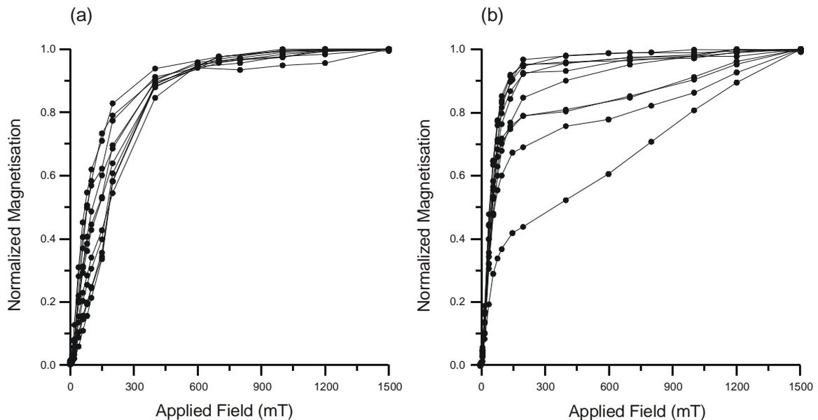
Figure 4-8: Normalized acquisition curves of a monodirectional isothermal remanent magnetization (IRM) in (a) sediments of the Klingler-Kar-Formation and (b) volcanics of the localities of Geisstein (GS) and Bischof (BF).
