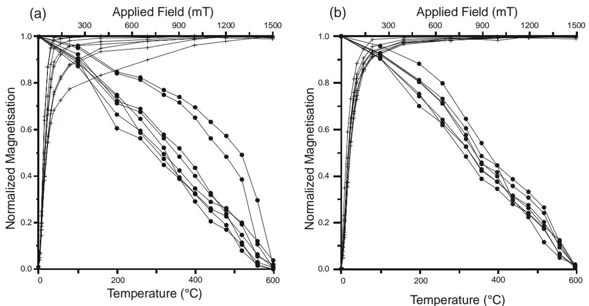
Figure 3-4: Normalised isothermal remanent (IRM) acquisition curves (crosses) and intensity decay plots of the subsequent thermal demagnetisation of the IRM (circles) for the Early Ordovician volcanic samples (a) and the Late Ordovician clastic sediments (b).
