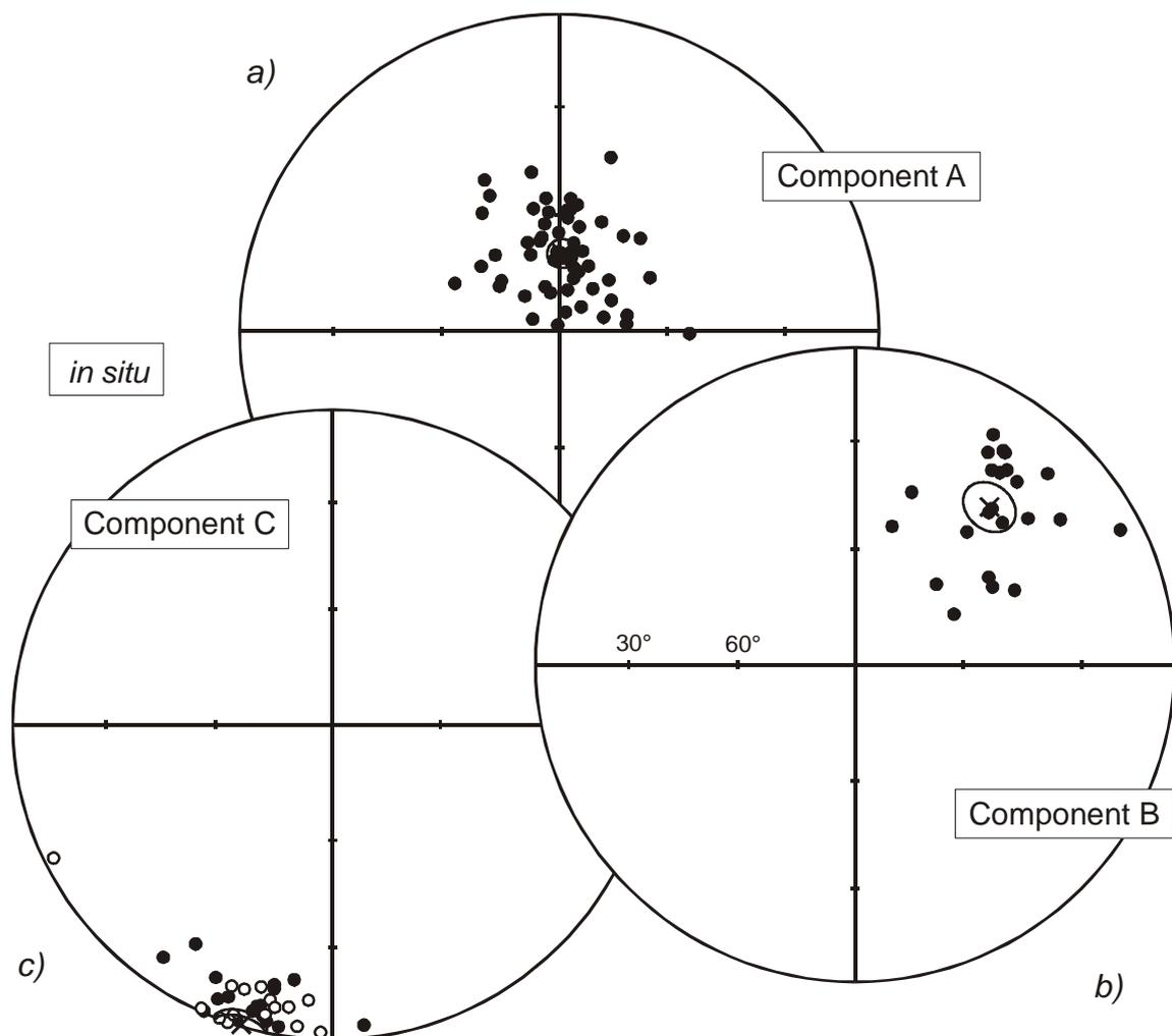
Figure 3-10: Equal area stereographic projection of thermal and alternating field demagnetisation results of samples of the Silurian Ockerkalk in geographic coordinates, in which straight line segments are identified. In (a) the component A, in (b) the component B and in (c) component C. Also shown is the cone of 95% confidence and the overall mean direction.
