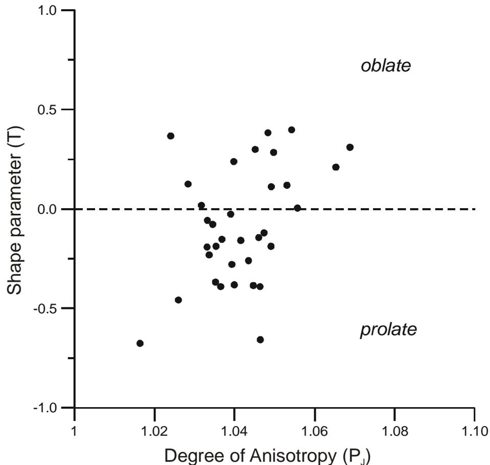
Figure 4-9: AMS fabric diagram for volcanics from GS and BF. The dashed line ( $T = 0$ ) represent an isotropic shape of the anisotropy ellipsoid.
