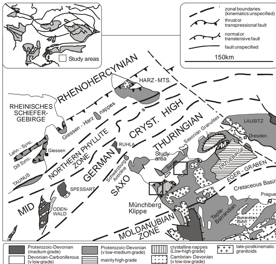
Figure 1-9: Simplified structural map of the main structural and lithological units within the Variscan fold belt of central Europe
