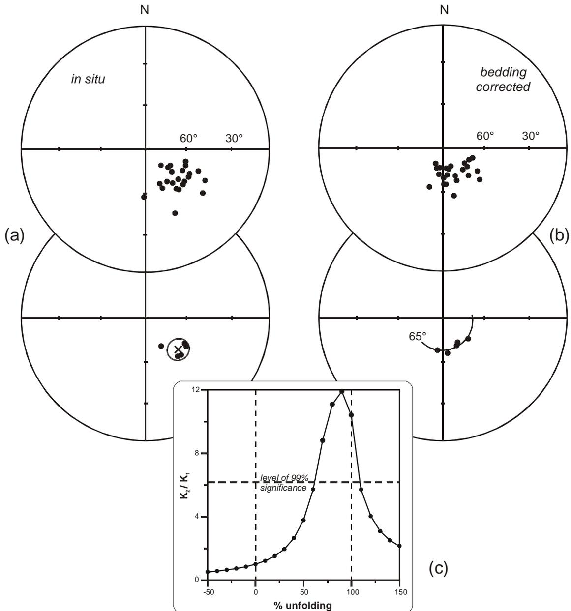
Figure 4-5: Equal area projection of the (a) in situ sample directions (above) and site mean directions (below), and (b) bedding corrected sample directions (above) and site mean directions (below) for component C along a small circle segment. (c) The calculated  $k_2/k_1$  ratio vs percentage of unfolding applying the inclination-only test. Notation as in Fig. 3.
