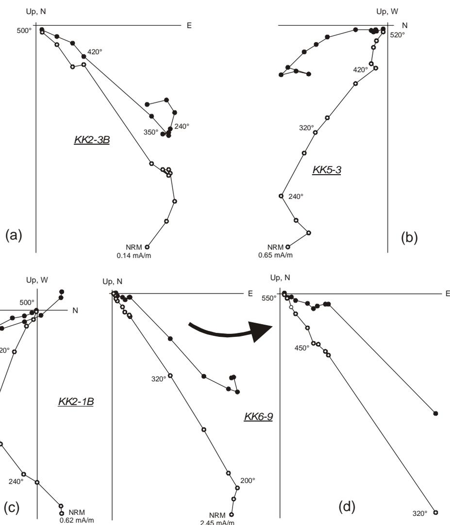
Figure 4-4: Orthogonal projection of typical thermal demagnetization results for the Upper Silurian sediments. All directions are plotted in situ, and solid (open) symbols represent the horizontal (vertical) component respectively. Temperatures are given in degrees Celsius. All samples show a removal of A up to 240°C, removal of B up to 450°C is obvious in sample (d). At temperatures higher than 420°C–450°C, C is identified as intermediate south-southeastward direction of magnetization.
