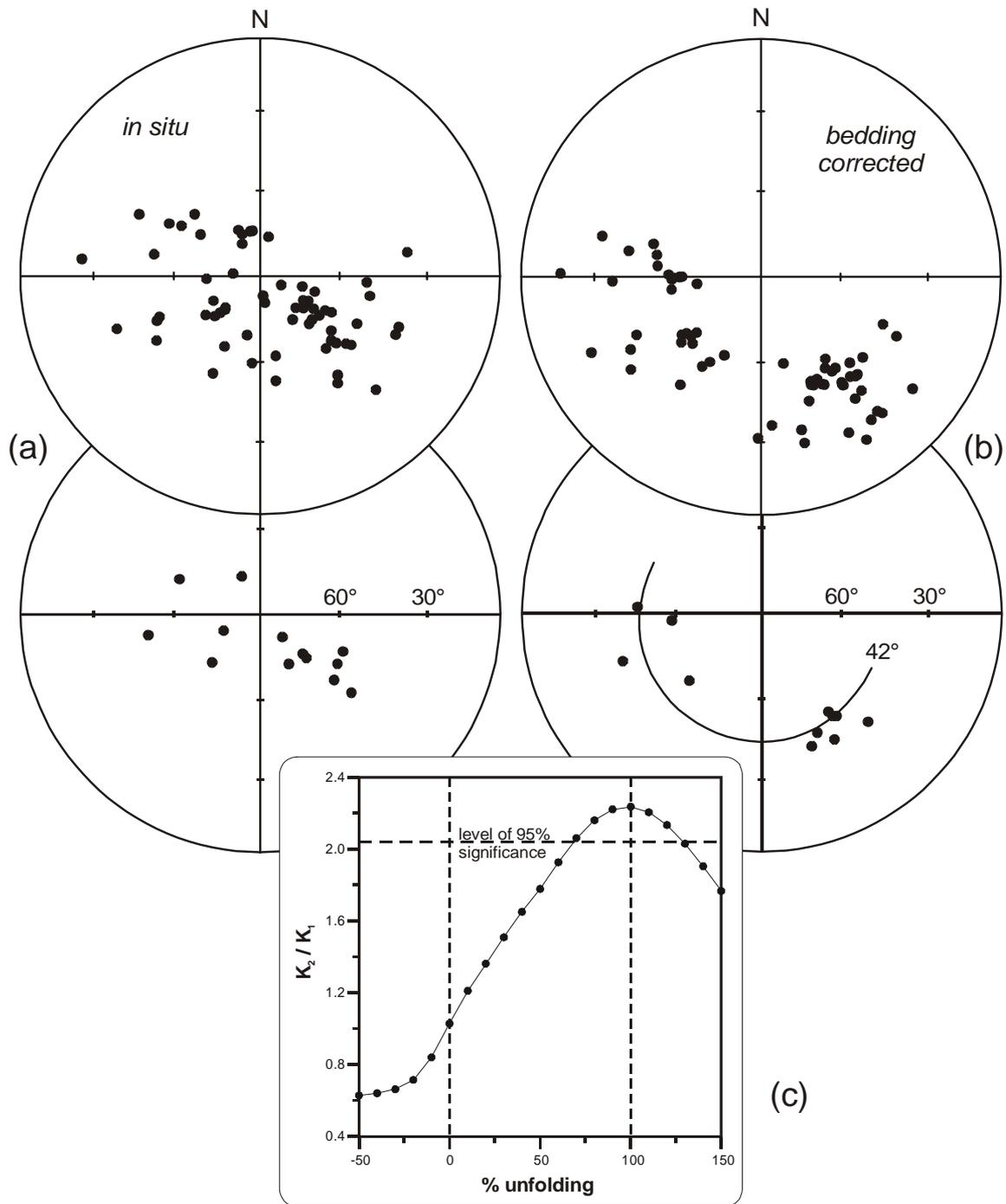
Figure 4-7: Equal area projection of the (a) in situ sample directions (above) and site mean directions (below), and (b) bedding corrected sample directions (above) and site mean directions (below) for component D along a small circle segment. (c) The calculated  $k_2/k_1$  ratio vs percentage of unfolding applying the inclination-only test. Notation as in Fig. 4-3.
