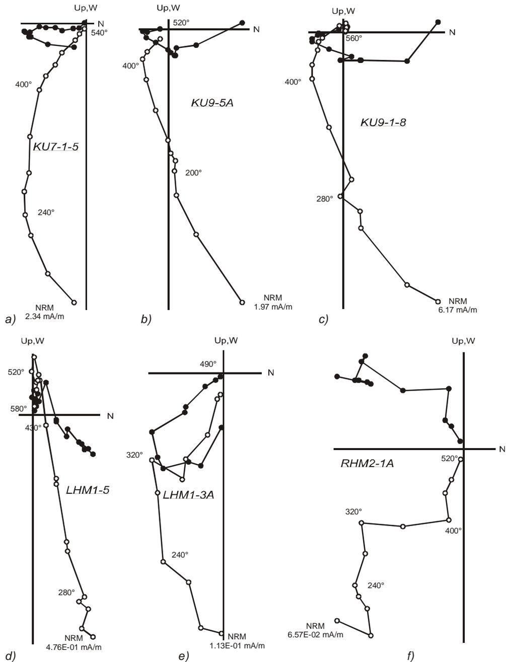
Figure 3-2: Orthogonal projection of thermal demagnetisation data for samples of the Early Ordovician volcanic samples (a-e) and the Late Ordovician clastic samples (f). Directions are plotted in situ, solid (open) symbols represent the horizontal (vertical) component, respectively.
