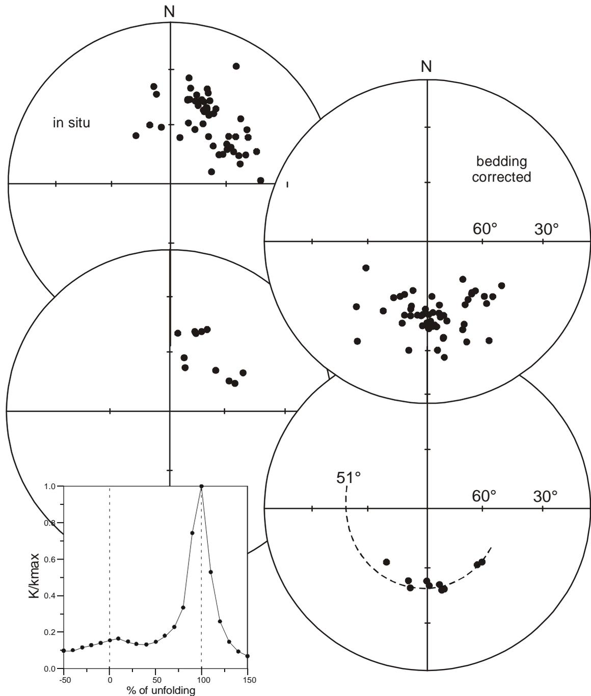
Figure 4-14: Equal area projection of the (a) in situ sample directions (above) and site mean directions (below), and (b) bedding corrected sample directions (above) and site mean directions (below) for component C2 along a small circle segment. (c) The calculated  $k/k_{max}$  ratio vs percentage of unfolding applying the inclination-only test. Notation as in Fig. 4-3.
