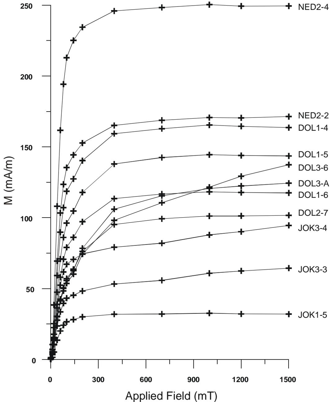
Figure 3-7: IRM acquisition curves of monodirectional isothermal remanent magnetisation
