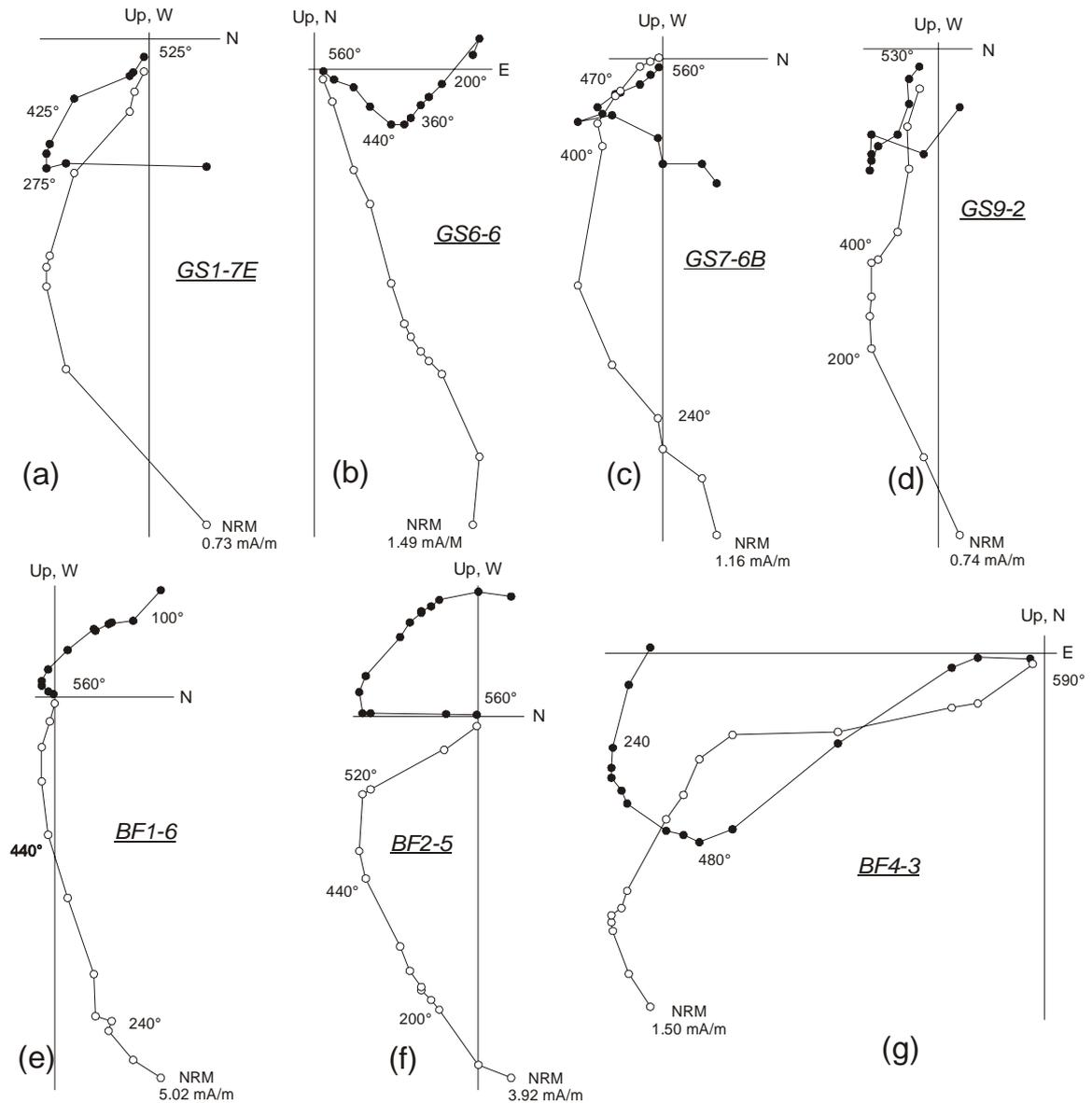
Figure 4-6: Orthogonal projection of thermal demagnetization data for samples from the Mid Devonian volcanics. All directions are plotted in in situ coordinates. Notation as in Fig. 4-4. Samples (a), (d), (e), (f), (g) show a removal of component A up to 200°-275°C. At intermediate temperatures up to 400°-440°C component B is removed in (b) and (c). At temperatures higher than 400°-480°C, the samples reveal the component D.
