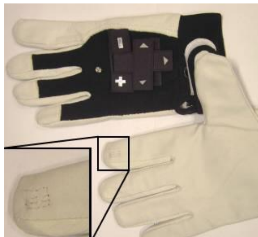
Figure 60: The prototypes used to demonstrate the idea of adding touch input on gloves. Some configurable buttons are placed on the left palm. The right index finger is used to initiate commands.
