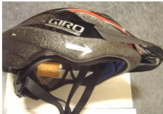
Figure 59: An off-the-shelf bicycle helmet equipped with touch sensitive areas on both sides ('GIRO' logo and the arrow). A lamp in the front can give feedback.
