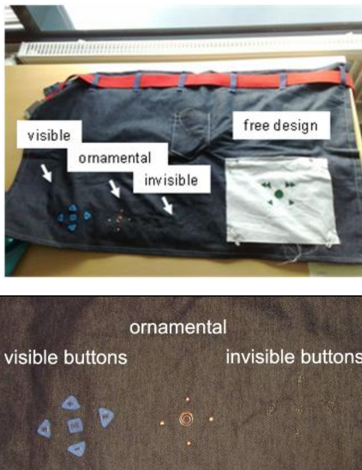
Figure 61: The apron ( top ) and close-up of the 3 different designs of the touch buttons ( bottom ).
