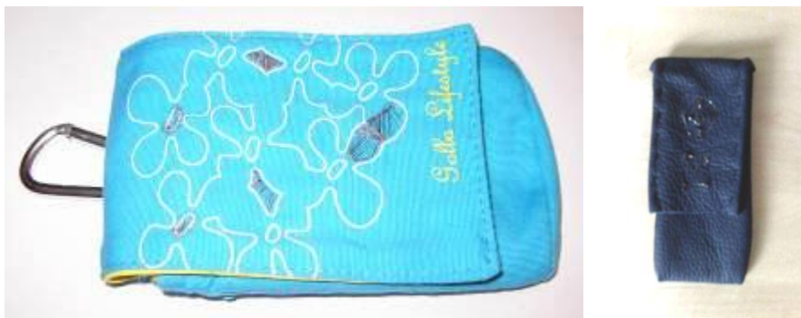
Figure 58: Left: One of the phone bags with five touch areas seamlessly integrated in the existing design. Right: a smaller phone bag with just two touch areas, ornamental and blackened, thus barely visible.
