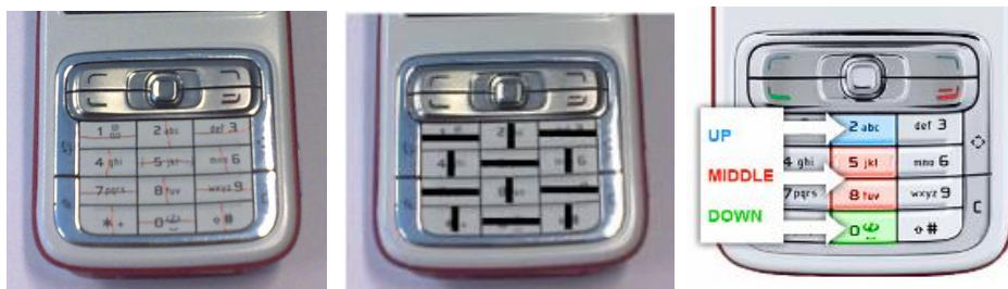
Figure 68: Layout of the electrode wires on the keypad of the N73 and its use in the test applications.
