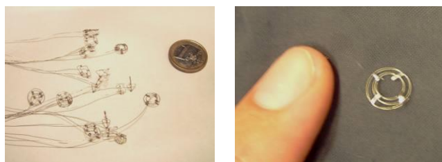
Figure 87: Prototyping material for quickly testing control interface layouts: several strips of conductive wires with ornamental buttons can quickly be connected to the sensing system.
