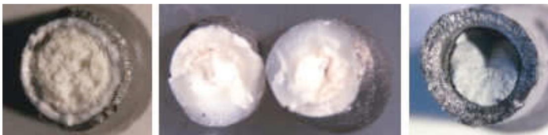
Figure 2.27: Left: Beginning reaction; Middle: Nearly complete reaction with the BN-crucible; Right: Complete reaction. [84]
