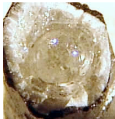
Figure 4.103: BN-crucible with glassy tin borate.
