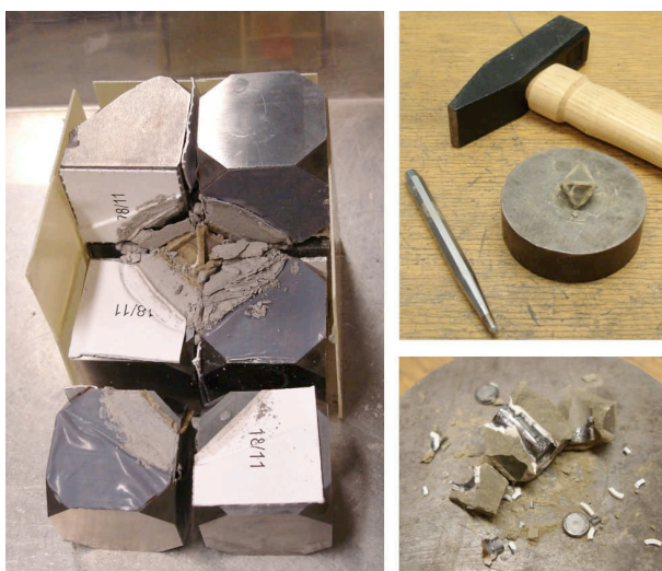
Figure 2.25: Left: Cube of inner anvils opened after a high-pressure/high-temperature program. Right, top: Hammer and centre punch to open the octahedron. Right, bottom: Opened octahedral pressure medium.
