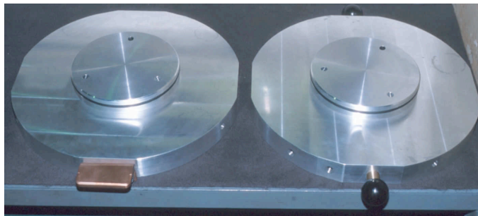
Figure 2.9: Pressure-distribution plates (left: bottom; right: top). [84]
