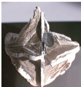
Figure 2.28: Recovered octahedron after a blow-out. [84]
