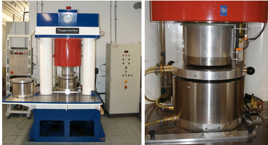
Figure 2.19: Left: Front view of the press with heating control (left) and press control (right). [51] Right: Walker-type module under the ram.
