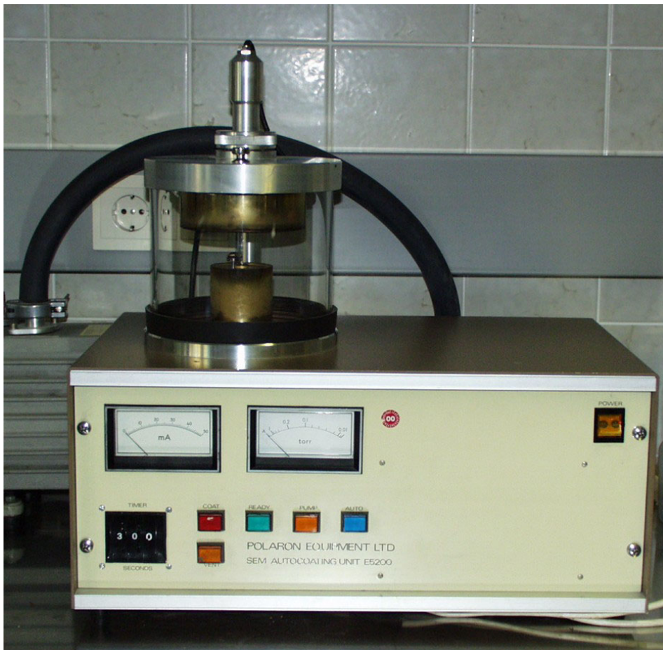
Abb. 9: Sputteranlage, SEM Autocoating Unit E5200, Polaron Equipment Ltd. - Quorum Technologies, Newhaven, England.
