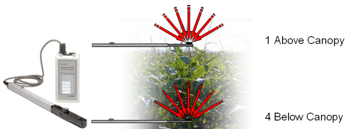
Figure 4.10: Principle of a leaf area measuring cycle with the LI-COR LAI-2000 instrument.
