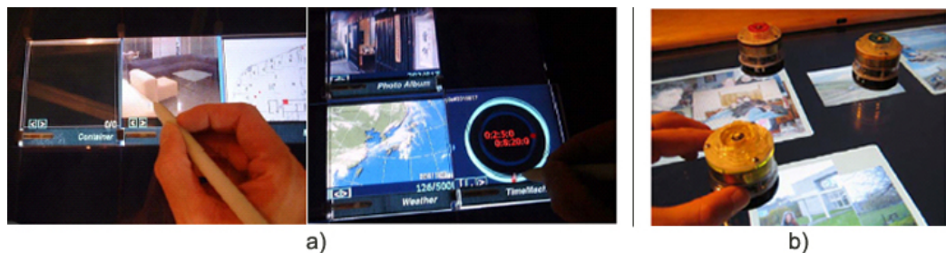
Figure 3.18: Examples of objects as tools for local modification: a) Interacting with DataTiles for editing the information displayed underneath, or aside a tile (Rekimoto et al., 2001); b) Using physical pucks for moving photos on TViews (Mazalek et al., 2006).
