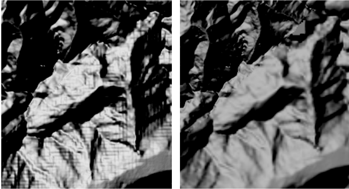
Figure 4.9: Artifacts in the data derived from the DTM. The images show a visualization of the cosine of the local solar incidence in an area where the 75m DTM of Tyrol (southeast section) abuts the 30m resolution DTM of Bavaria (northwest section). In the left image, the calculation was performed on interpolated data at 30m. In the right image the calculation was performed on the 75m data and the local solar incidence angle was interpolated and merged with the 30m data.
