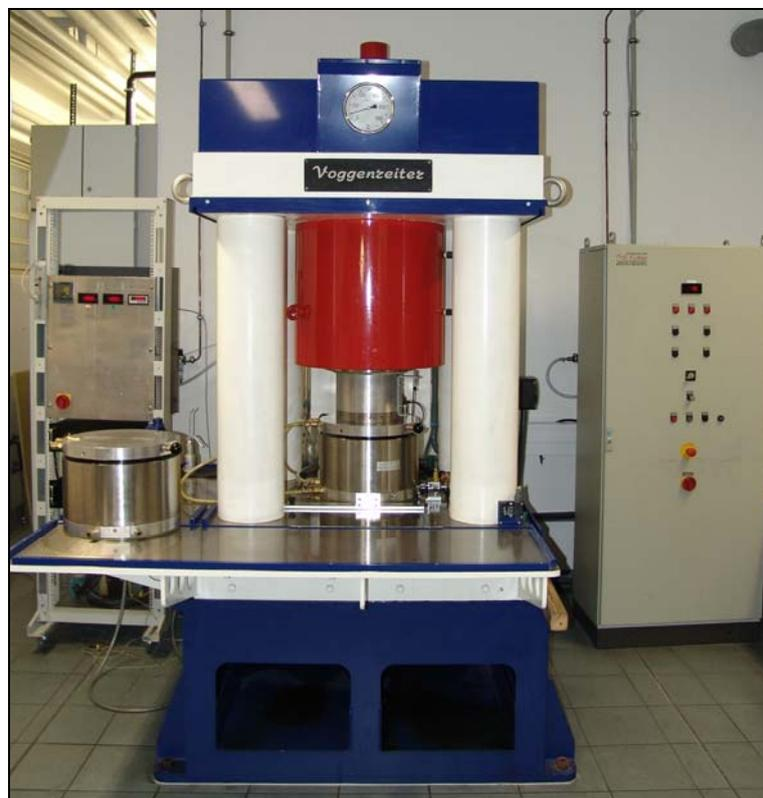
Figure 2.2-1: 1000 t press with heating- (left side) and control-unit (right side).
