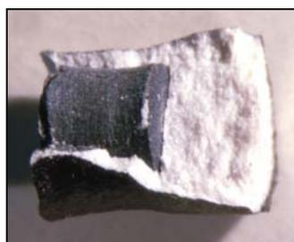
**Figure 2.2-35:** Intermetallic phase in a BN capsule [30].
