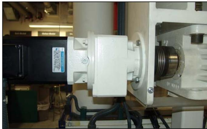
**Figure 2.2-12:** Servomotor for slow pressure changes.
