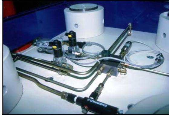
**Figure 2.2-10:** Hydraulic valves and oil pipes on the top plate of the 1000 t-press [30].
