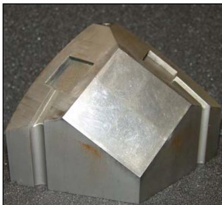
**Figure 2.2-3:** Single tool steel wedge with wiring channels.
