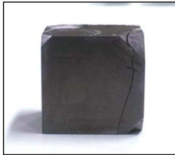
**Figure 2.2-38:** WC cube with crack [30].
