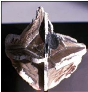
**Figure 2.2-37:** Octahedron after a blow-out [30].
