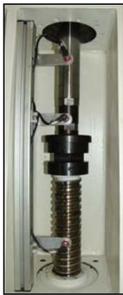
**Figure 2.2-11:** Worm gear screw jack
