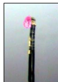
**Figure 4.1-5:**  $\alpha$ -Nd<sub>2</sub>B<sub>4</sub>O<sub>9</sub> crystal on a glass fiber.
