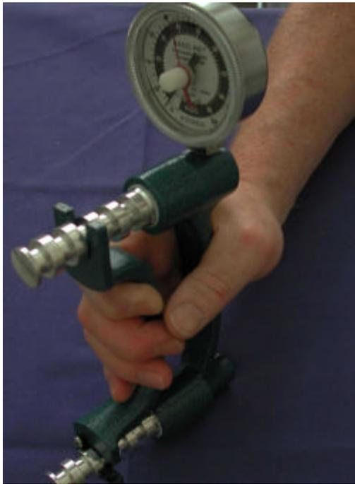
Abb. 6, Baseline Hydraulic Hand Dynamometer
