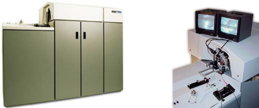
Figure 1.27: Depiction of components of a mass spectrometer: a) Qstar pulser quadrupole mass analyzer, b) ion-spray source
