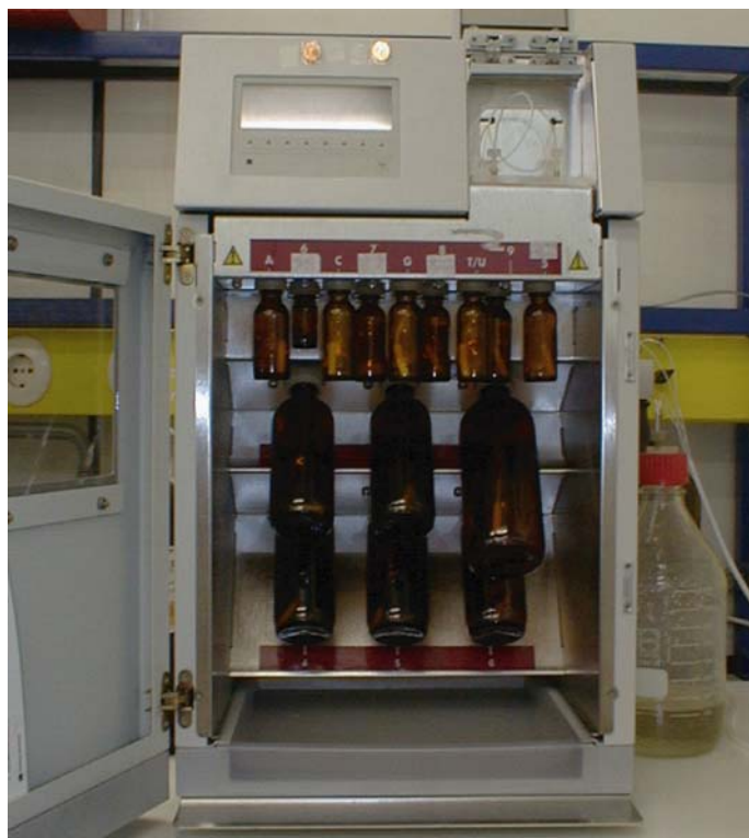
Figure 5.1: Depiction of a Perseptive Biosystems' Expedite™ 8900 automated DNA synthesizer used in this study for automated DNA-synthesis.
