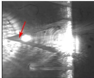
**Figure 8: Alignment of the AFM laser onto the gold-coated back surface of the cantilever. The red arrow indicates the position of the laser focus on the shank.**
