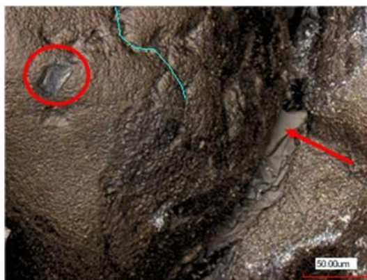
Figure 4.4 Grain surface and pore throat of sample RL I_4146 imaged by CLSM at 50x magnification. The surface of the grain is sculptured by micro-pits (line mark) and overgrown by authigenic minerals (circle). The pore throat is blocked by cement filling (arrow).
