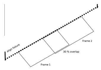
**Fig. 2.** Acquisition scheme for the sampling of roughness measurements with a given length and its components using a single reference frame.
