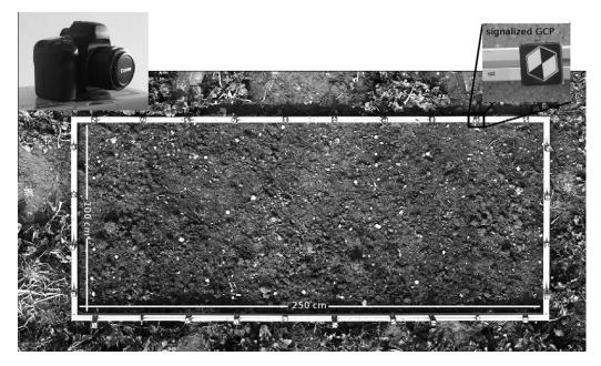
Fig. 1. Reference frame for relative orientation of the images acquired for DSM generation and detailed view of a GCP.
