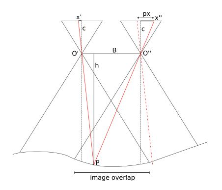
Figure 1.8: Photogrametric object reconstruction with x' = x-parallax in the left image; x'' = x-parallax in the right image; px = x'-x''; B = Base; h = mean lens height above ground; O = projection center;
