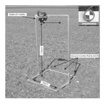
**Fig. 3.** Camera system for photogrammetric image acquisition (setup and signalized control point).
