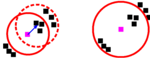
Figure 3.13: A schematic illustration of the effect that by increasing the bandwidth new clusters can appear.
