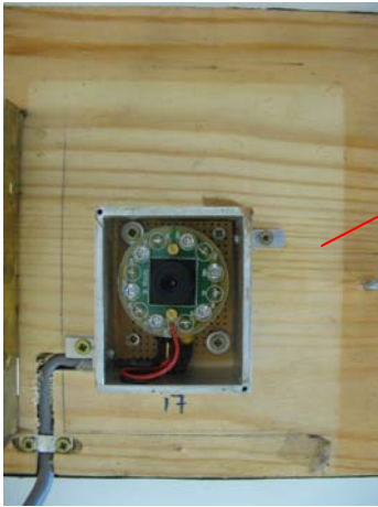
Fig. 1a Mini-camera attached to the inside of a nestbox lid, surrounded by six infrared light LEDs
