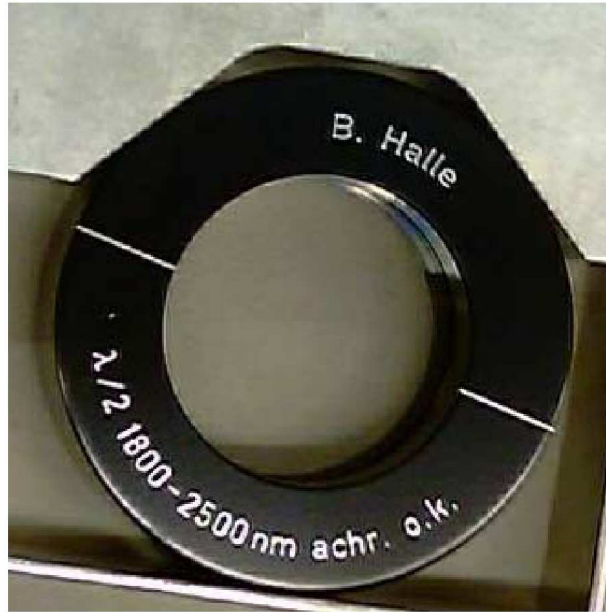
Figure 4.8 Half-wave plate (provided by Bernhard Halle Nachfl ) in a test mount.
