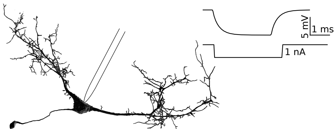
Figure 4.1: Illustration of a simulation of a current clamp experiment to calculate input resistance ( R_{in} ) and effective membrane time constant ( \tau_{eff} ) of a multi-compartmental model.
