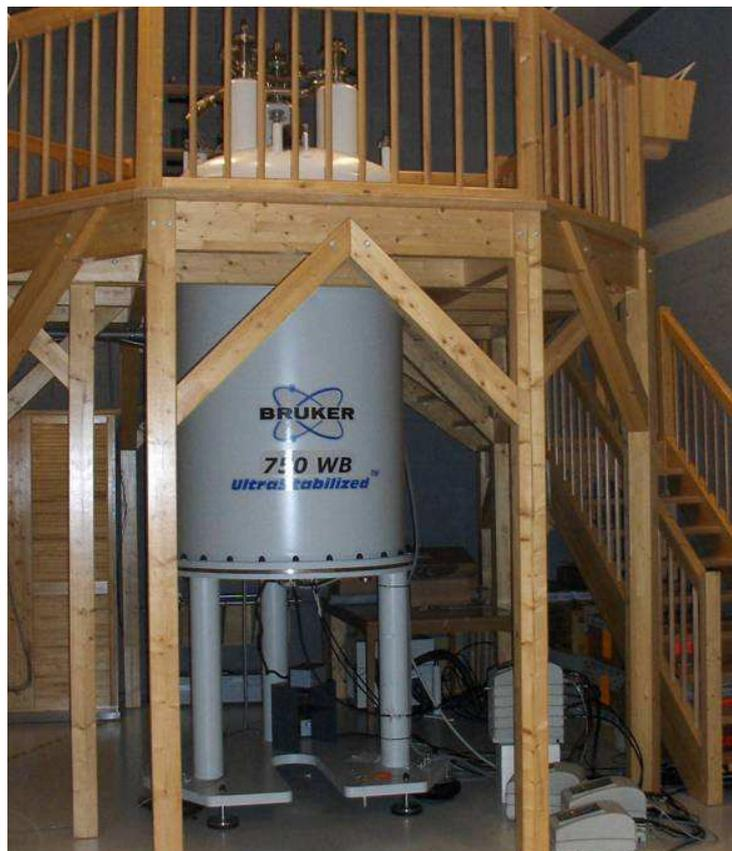
Figure 5.1: A 17.6 T magnet (Bruker Biospin GmbH, Rheinstetten, Germany) was used for the MRI experiment. Its main magnetic field was oriented perpendicular to the floor (vertical).
