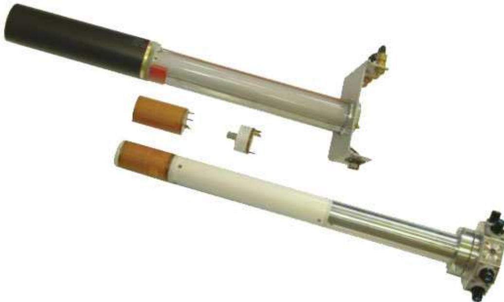
Figure 5.2: Micro 2.5 gradient system (top), probe body (bottom) and exchangeable resonator (middle).
