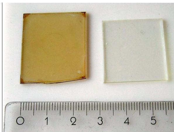
**Figure 3.8:** Films on glass slides as-synthesized H-D1-100 °C (right) and H-D1-400 °C after pyrolysis at 400 °C (left).
