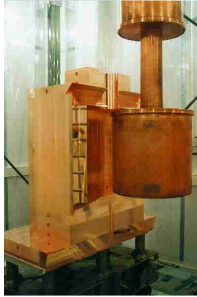
Figure 2.2: Picture taken while remounting the CRESST experiment in Hall A. The cold box together with the copper shielding is shown. The outer lead shielding was not yet mounted.
