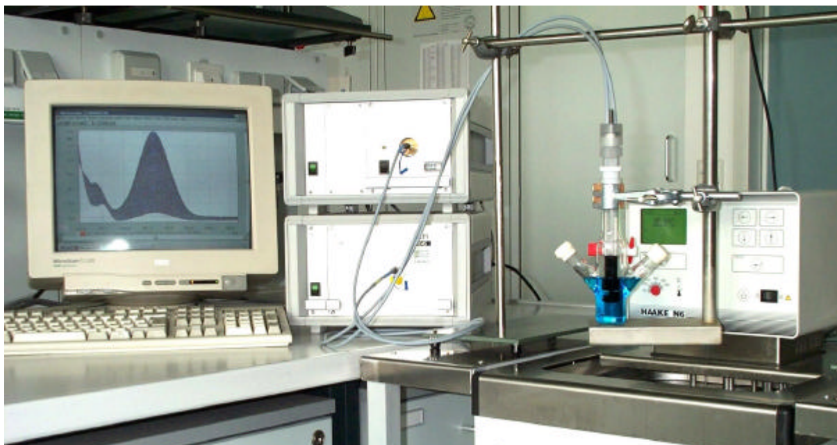
Figure 2.1: J&M TIDAS diode array spectrometer connected to Hellma 661.502-QX quartz Suprasil immersion probe via fiber optic cables.
