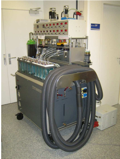
Figure 5 The Olfactometer (OM6b, Burghart).
