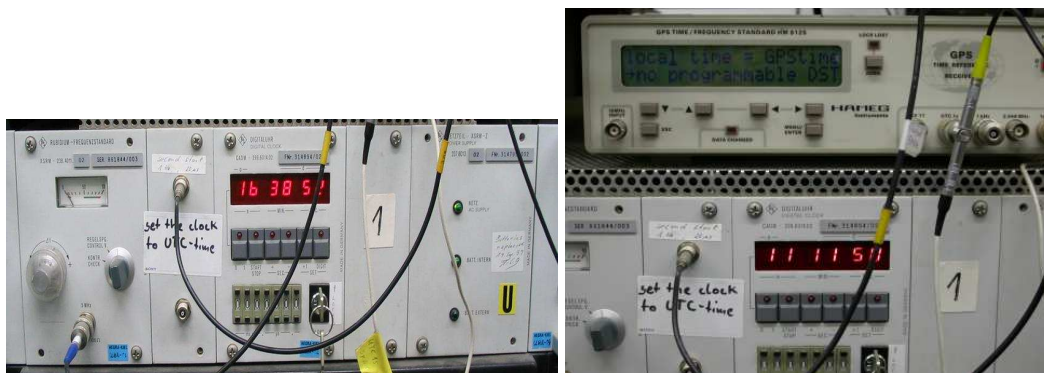
Figure 3.25: Left: A photograph of the rubidium clock, adopted from [214]. Right: A photograph of the GPS clock on top of the rubidium clock, adopted from [214].
