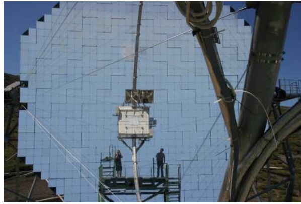
Figure 3.12: A photograph of the reflector adopted from [214]. Square shaped mirror panels can be seen.
