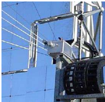
Figure 3.23: A photograph of the pyrometer adopted from [214]. It is installed at the edge of the reflector.
