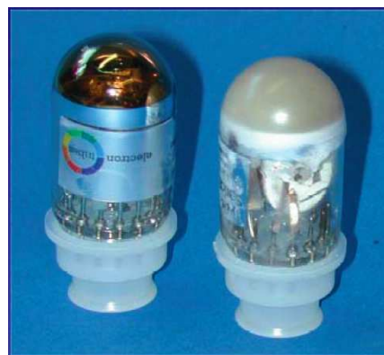
Figure 3.14: Left) Passively enhanced QE curve of PMT ET9116, overlaid with Cherenkov radiation spectrum and NSB spectrum (not in scale). The QE curve is well optimized for the Cherenkov radiation. A hump at 280 nm is due to the wavelength shifter coating. Right) Photograph of PMTs, before (left) and after (right) the diffusive coating.
