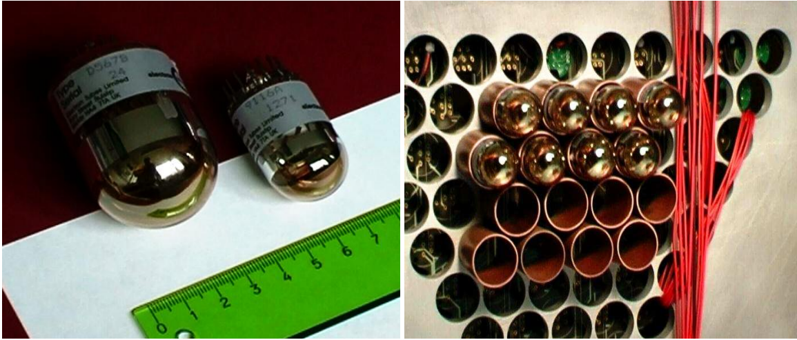
Figure 4.5: The left picture shows two different sizes of the PMT pixels used in the MAGIC telescope. The right picture shows the PMT pixel module in the camera plane.
