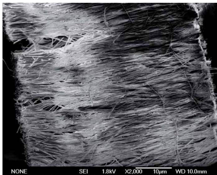
Figure 3.5 — SEM image of mesoporous organosilica filaments templated within anodic alumina pores. The alumina mold has been etched to obtain free filaments.
