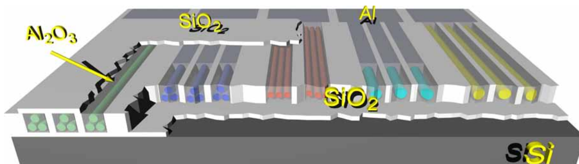
Figure 5.1 — Schematic of a multi-contact horizontal anodic aluminum oxide device. Due to separation of the Al contacts, anodic microscopic finger ensembles can be anodized individually, enabling the fabrication of a horizontal porous alumina structure containing different pore morphologies, i.e., different pore diameter, interpore distances, and pore length. The resulting composite can then be used for the subsequent growth of nanowire arrays. Due to the electrical insulation of the individual contacts it is possible to grow different nanowires of different compositions (as indicated by the different colors of the wires in the above scheme) on the same chip.
