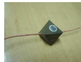
Figure 2-28. Prepared octahedron for the temperature calibration.
