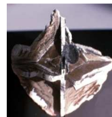
Figure 2-20. Octahedron after blow-out [109].
