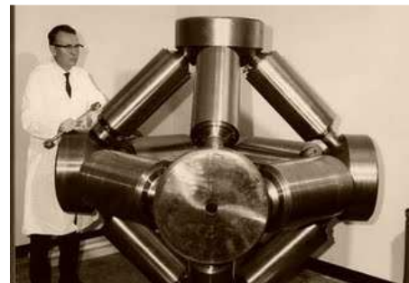
Figure 1-3. T. Hall with tetrahedral press [23].
