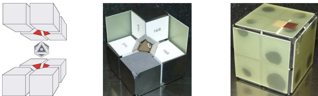
Figure 2-14. Insertion of the octahedron into the eight tungsten carbide cubes (inner anvils) [66,109].
