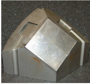
Figure 2-8. Single tool steel wedge with wiring channels for calibration [109].
