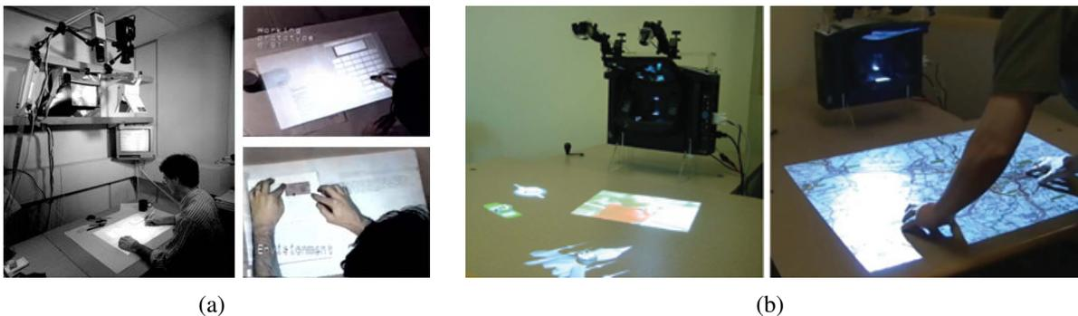
**Figure 6.4:** (a) Wellner's DigitalDesk setup on the left. Example applications include a projected calculator alongside a printed spreadsheet and copying printed information through simple gestures. (b) PlayAnywhere's compact and mobile setup. Bi-Manual map manipulations enabled by optical flow motion estimation.
