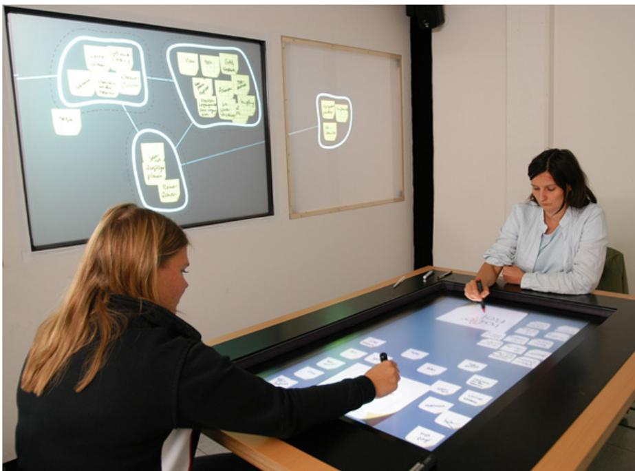
**Figure 3.1: Overview of the physical setup in Brainstorm. Smartboards embedded into the table and wall function as primary input surfaces. In the periphery additional interactive displays can be used to store information not currently used. A custom user interface has been implemented mimicking paper-based brainstorming but enhancing the technique through additional functionality invoked through gesture-based interaction.**
