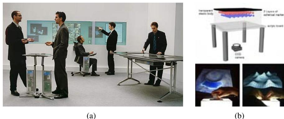
**Figure 6.7:** (a) SmartBoards and other direct-touch enabled surfaces in the **i-Land** project. (b) **GelForce** sensing principle and visualizations of the force-field produced by tangible objects and multiple hands interacting with the sensor.
