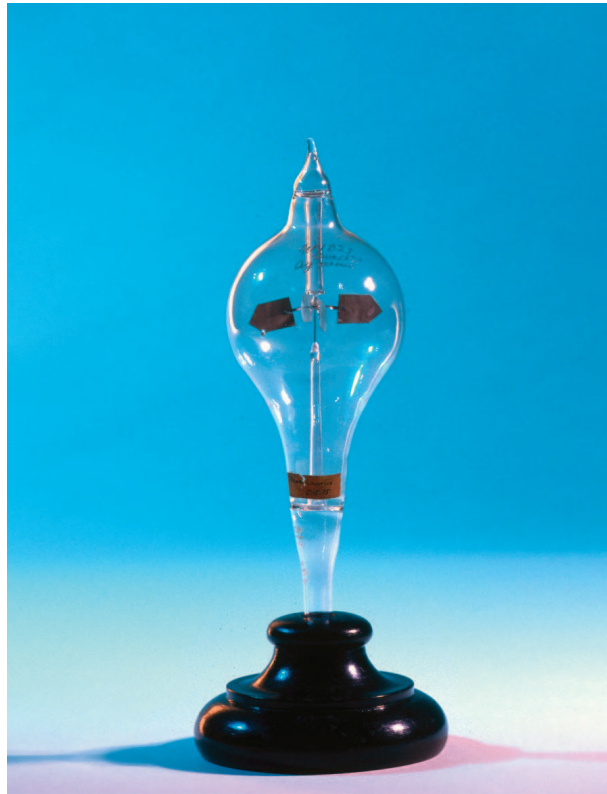
Figure 2.1: Radiometer used by Crookes around 1877. The pivoted vanes, each silvered and blackened on one face, are free to revolve around the central axis. Crookes observed that the vanes started to turn when illuminated by a strong light source. The origin of the effect was not radiation pressure, it was mediated by the dilute gas still present in the globe. In refined experiments by Lebedev in Russia and Hull in the US, effects of radiation pressure on mechanical objects were observed at the beginning of the 20 th century. Image copyright Science Museum/SSPL, London.
