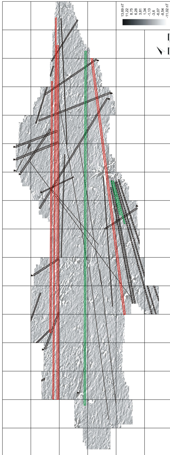
Figure 6.6. Interpretation of the geograph complex on site PP01-36 “Llipata” plotted on the Horizontal Gradiometer Mode magnetogram; SMARTMAG SMAG-Special in duo-sensor configuration; dynamics +/- 13 nT in 100 greyscale values from black to white (with 50% of transparency applied), sampling density 100 x 12,5 cm, interpolated to 25 x 25 cm, resolution increased by ‘Graduated Shade’ function; Earth’s magnetic field ca. 25000 nT; grid size 40 x 40 m;
