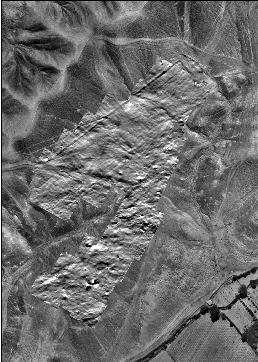
Figure 7.7. Magnetogram of the site PV67A-15/16 “Yunama” superimposed on the orthophoto of the same area; Caesium SmartMag SM4G – Special applied in the duo-sensor configuration. Sampling rate 12,5 x 50 cm interpolated to 25 x 25 cm, grid size 40 x 40 meter, dynamics +/- 7 nT, Earth’s magnetic field ca. 25.000 nT; orthoimage by K. Lambers, Institute of Geodesy and Photogrammetry, ETH Zurich, Switzerland.
