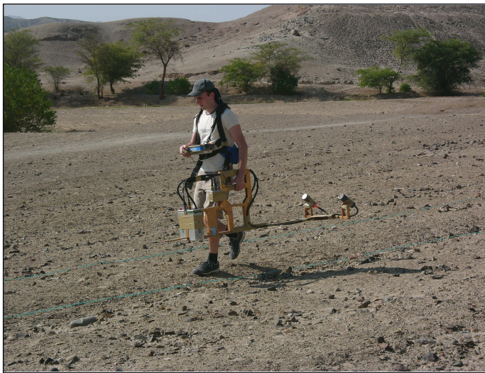
Figure 5.5. Field measurement in Palpa, southern Peru; March 2006; magnetic sensors' correction 45°.
